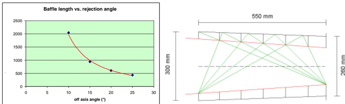
Fig. 2. LI Baffle sizing and design.
