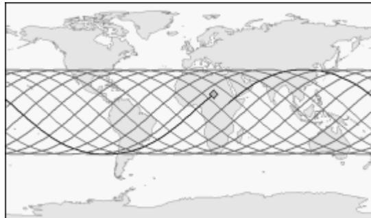
Fig. 8. The LIS field-of-view and the orbital track of the TRMM satellite during a 24 hour period (NASA).
