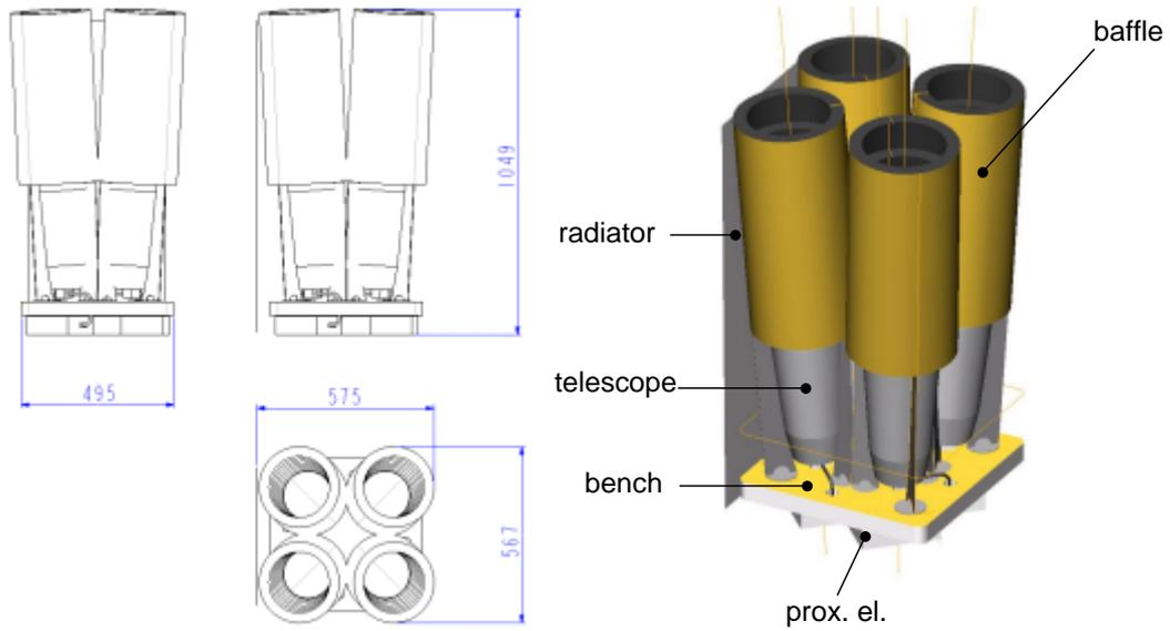
Fig. 3. MTG - Lightning Imager layout, sizing in mm.
