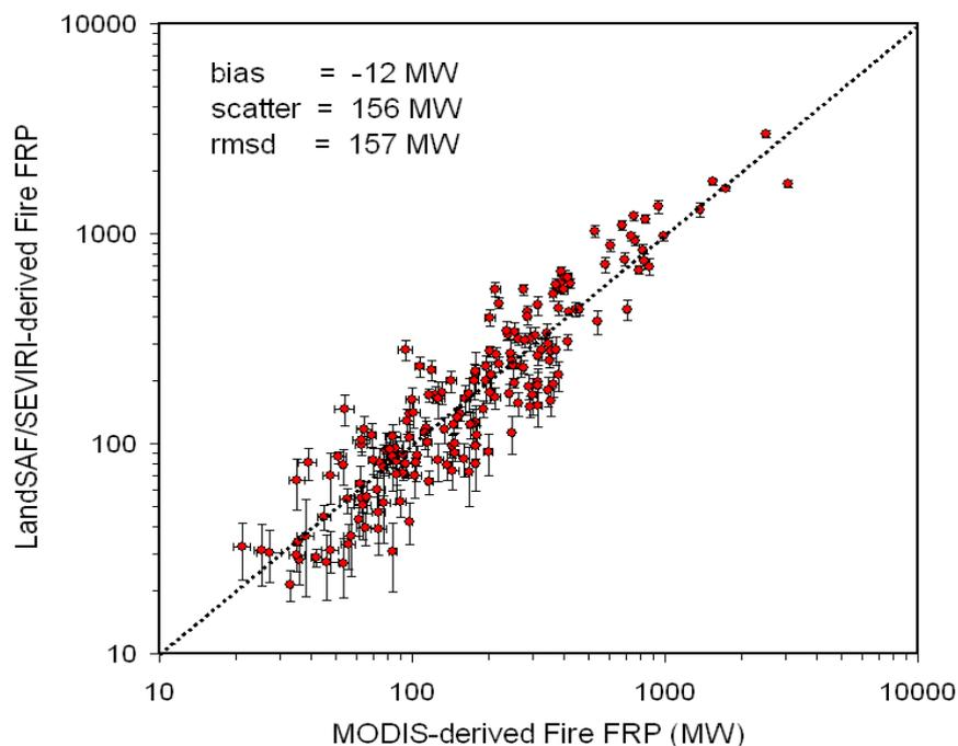
**Figure 4: A comparison of per-fire FRP derived from SEVIRI and MODIS observations of 187 fires observed near-simultaneously by each sensor. Fires are designated as contiguous clusters of active fire pixels and SEVIRI FRP measured were taken from the Land SAF FRP per-pixel products of southern Africa collected in August 2007.**
