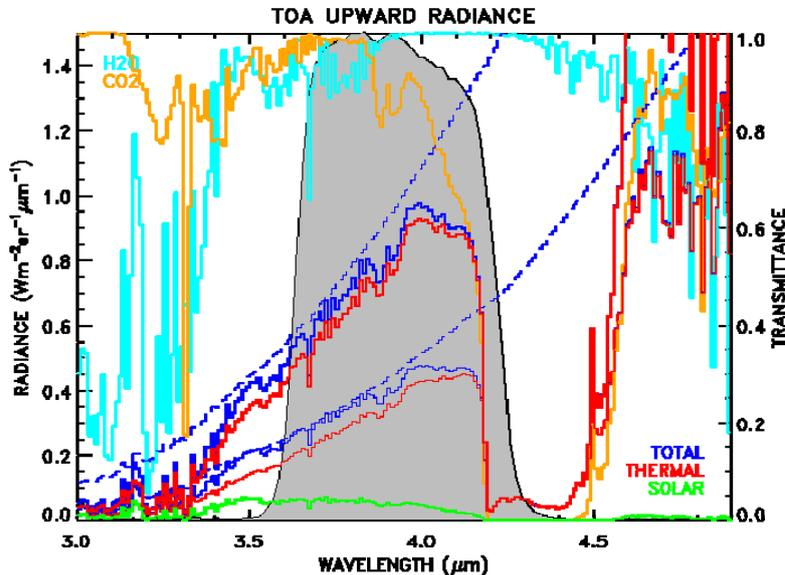
**Figure 3: Spectral response of SEVIRI 3.9  $\mu\text{m}$  band (shaded grey) shown for two different pixel temperatures. The dashed line is the total surface radiance, the solid blue line is the total TOA radiance, the solid red line is the thermal TOA radiance, the green line is the solar TOA radiance. The brown (light blue) line is the total  $\text{CO}_2$  ( $\text{H}_2\text{O}$ ) gaseous transmittance.**
