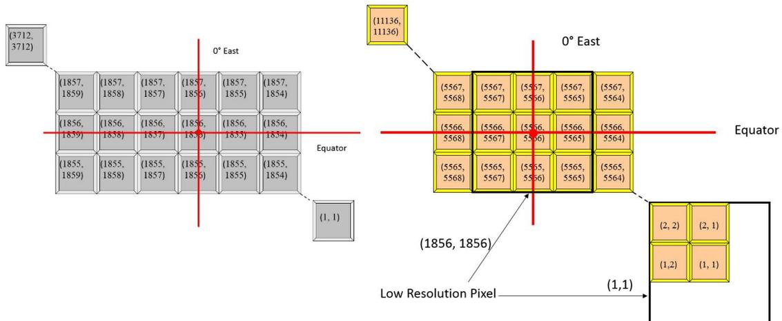
**Figure 2:** METEOSAT Second Generation SEVIRI level 1.5 images. Left: low resolution grid (3km SSD), right: high resolution grid for HRV images (1km SSD).
