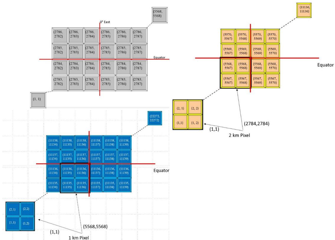
**Figure 3:** METEOSAT Third Generation FCI level 1c images. Top left: low resolution grid for 2 km SSD, top right: 1 km SSD grid, bottom left: high resolution grid for 0.5 km SSD.
