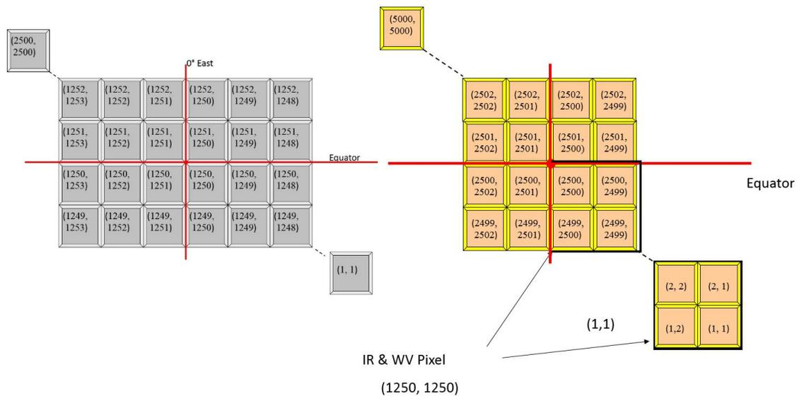
**Figure 1:** METEOSAT First Generation MVIRI rectified images. Left: low resolution grid for IR and WV images (4.5 km SSD), right: high resolution grid for VIS image (2.25 km SSD).
