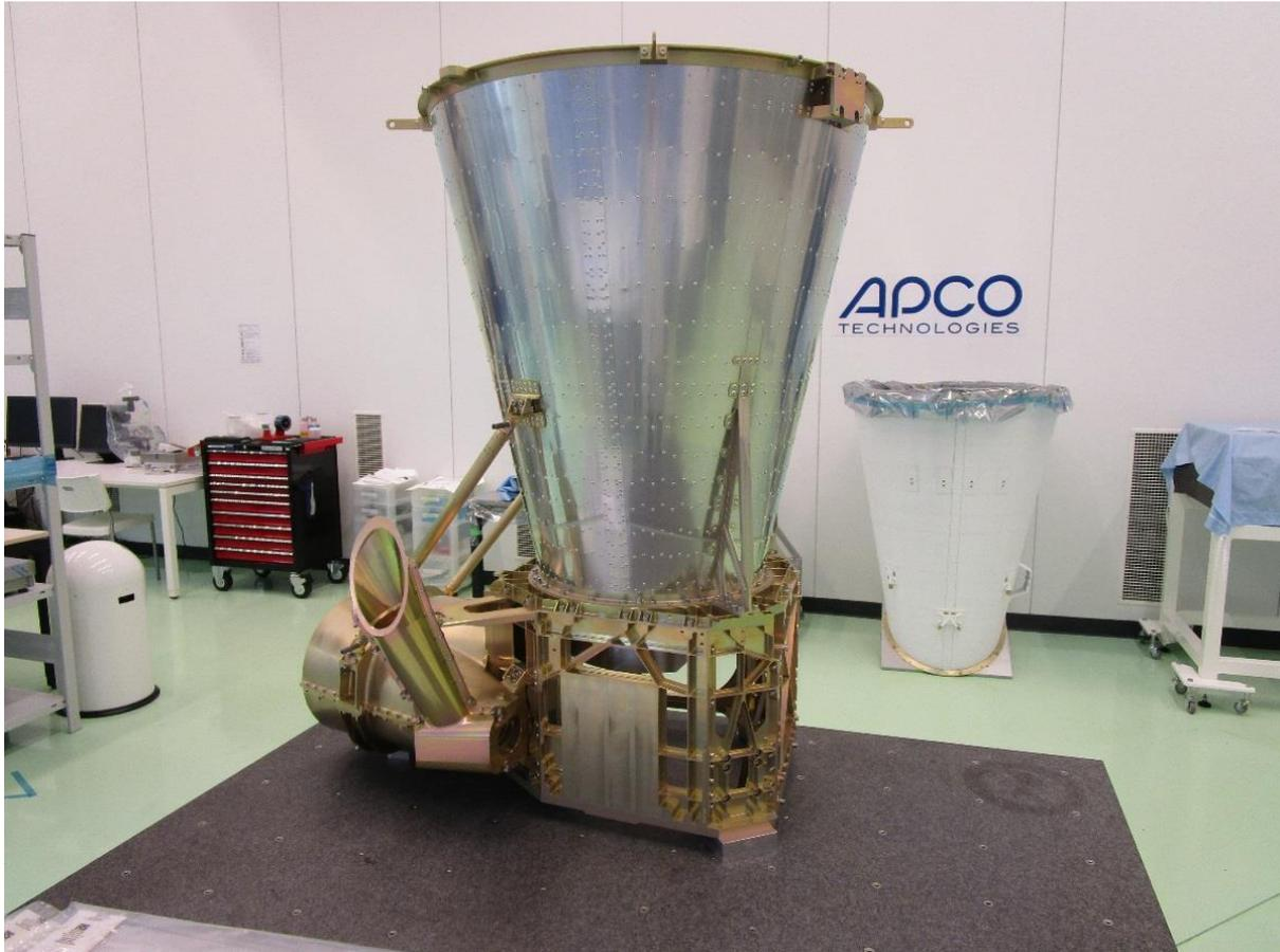
**Figure 1: IRS Entrance Baffle**
