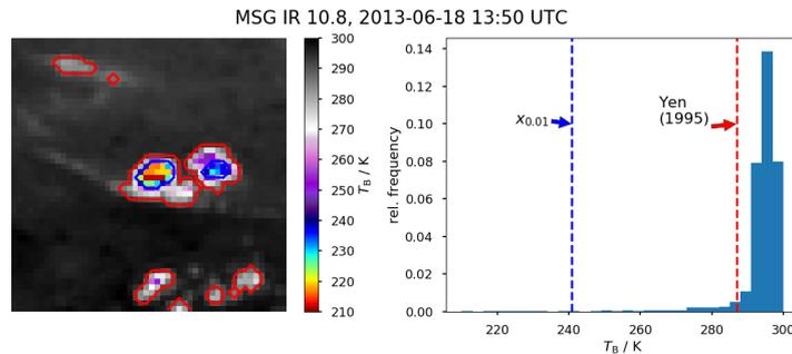
**Figure 3:** Principle of the hysteresis thresholding used for the object tracking method. Taking two thresholds (red and blue lines in the left panel and contours in the right panel), the image is segmented into background and objects.
