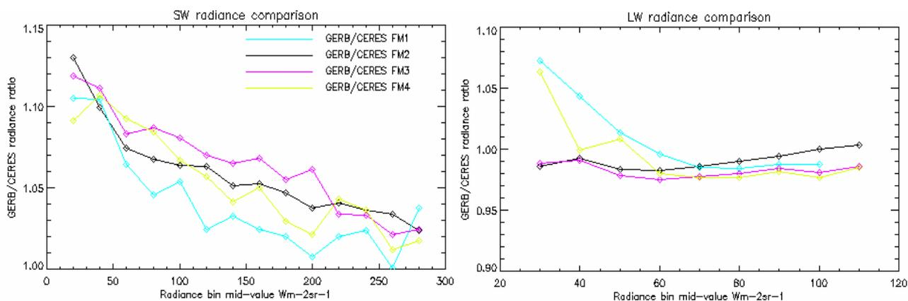
**Figure 1.** GERB/CERES radiance ratios for each of the four CERES instruments as a function of GERB radiance. Ratios determined from average GERB and averages CERES observations in each radiance bin. SW radiance comparison results are shown in the left hand panel and LW radiance comparison results in the right hand panel.
