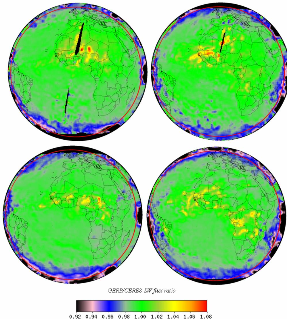
**Figure 3.** LW flux comparison for June (left) and December (right). GERB/FM2 ratio shown for day-time matches in upper panels and night-time matches in lower panels. Ring in red shows limit of VZA = 70°
