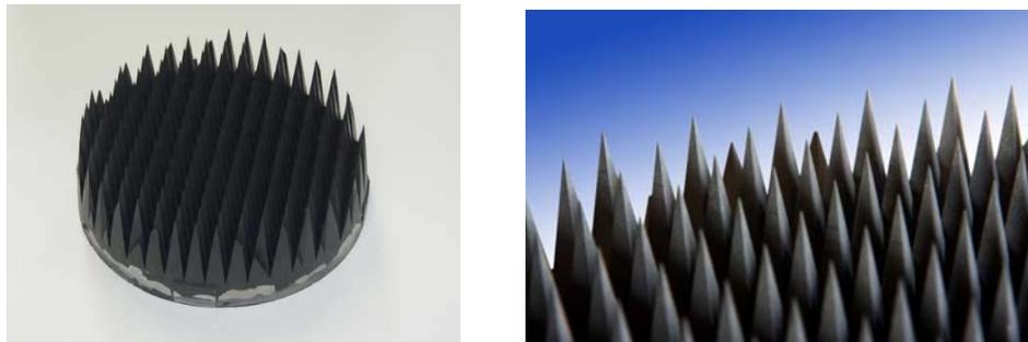
Figure 8: RAL Calibration Target (left) and Close-Up of Tip Geometry (right)
