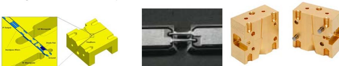
Figure 7: 664GHz Mixer design (left), RAL diode chip (centre) and machined block (right)
