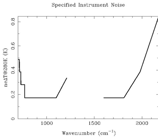
**Figure 5:** MTG-IRS specified instrument noise.
