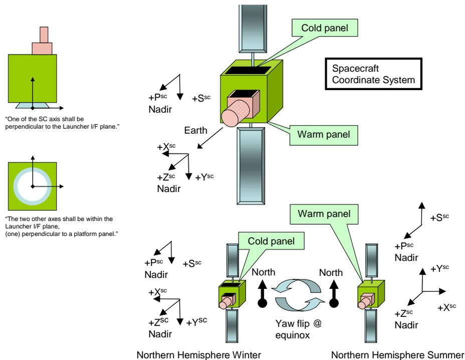
**Figure 2: MTG dual wing configuration and coordinate system**
