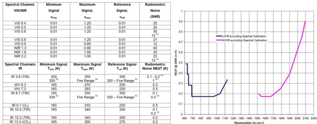
Figure 5: Radiometric noise requirement for FCI and Noise template for IRS.
