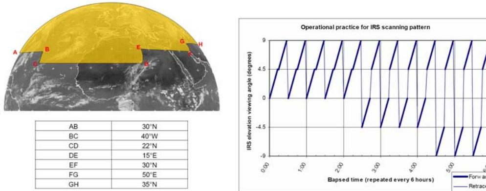
Figure 4: MTG IRS operational scenario scanning pattern
