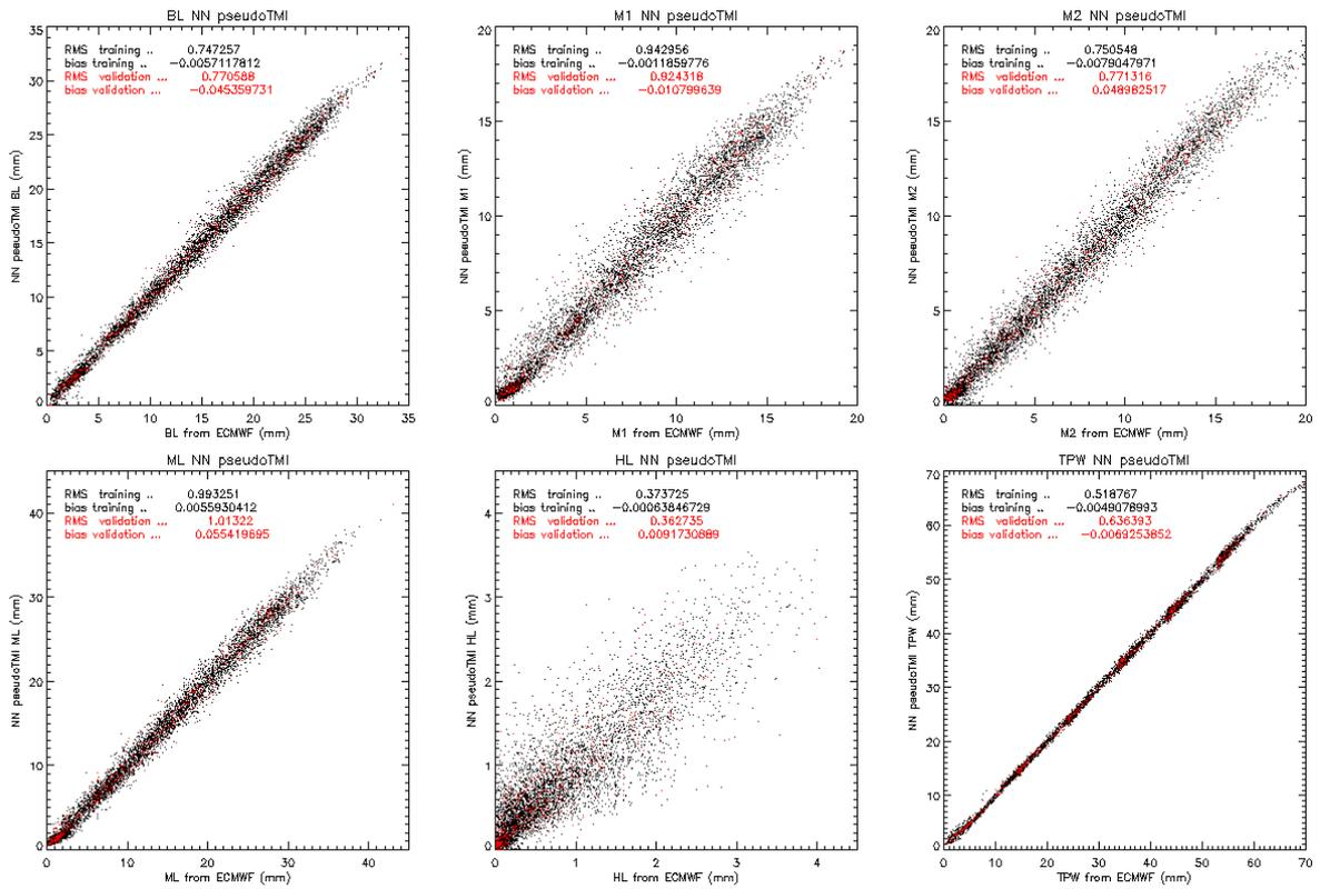
Figure 2. TPW and LPW scatter plots for the pseudo-TMI model (use only of TMI channels as Proxy for GMI). From left to right and top to bottom BL, M1, M2, ML, HL and TPW scatter plots. Red dots are from validation datasets, black dots are from training dataset.
