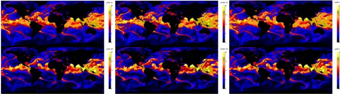
**Figure 8.** New M1 Layer (top) and M2 Layer (bottom) comparison. Calculated from the ECMWF profiles (center); using pseudo-TMI (left) and from pseudo-GMI neural network (right). 17th September 2006 at 12 UTC.
