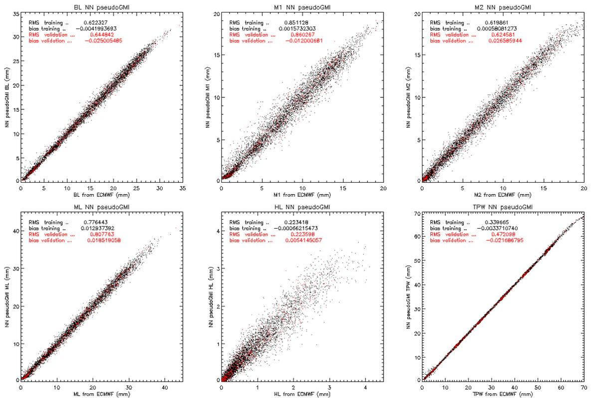
Figure 3. TPW and LPW scatter plots for the pseudo-GMI model (TMI channels and 3 channels from MHS as proxy for GMI). From left to right and top to bottom BL, M1, M2, ML, HL and TPW scatter plots. Red dots are from validation datasets, black dots are from the training dataset.
