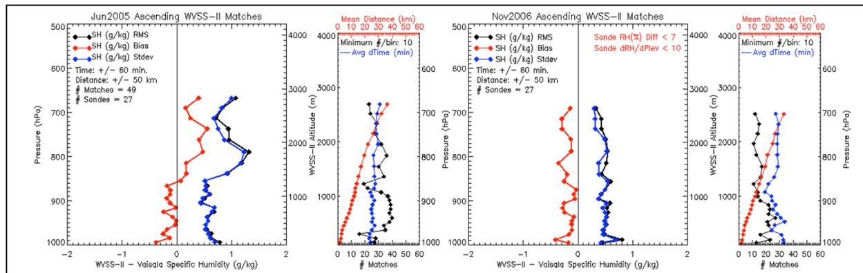
Figure 2 - Comparison of WVSS-II performance statistics by vertical level for 2 week periods in Spring 2005 (left) and Fall 2006 (right). Display content similar to Figure 1.
