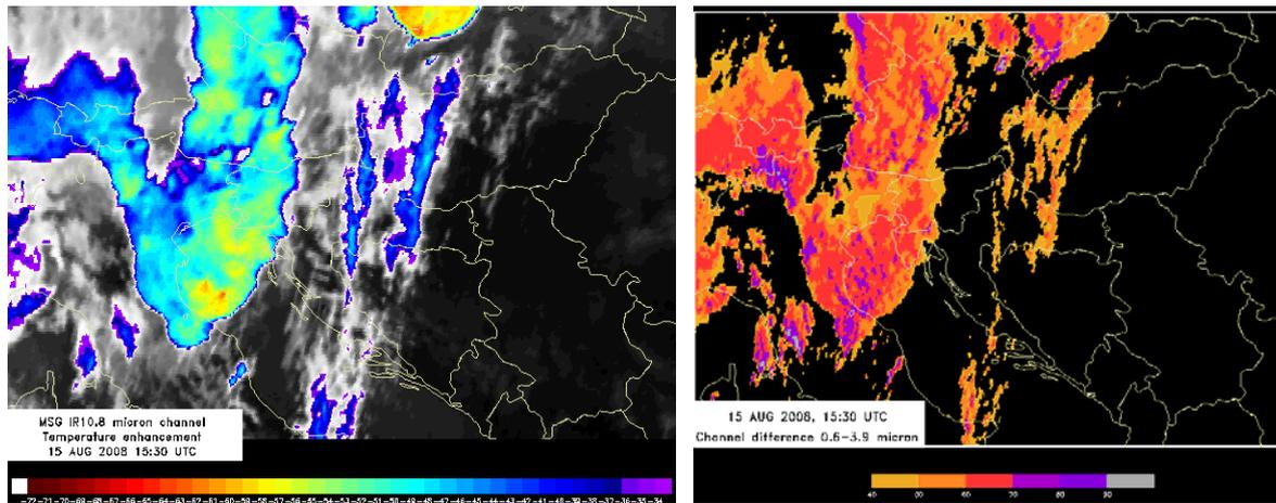
**Figure 4:** Meteosat-9 images for 15 August 2008 at 15:30 UTC: colour-enhanced IR10.8  $\mu\text{m}$  image (left) and the difference of reflectance in 0.6 - 3.9  $\mu\text{m}$  channel (right).
