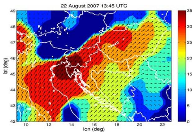
**Figure 3:** Cloud motion vectors for 22 August 2007 at 13:45 UTC based on Meteosat-9 IR10.8  $\mu\text{m}$  channel data. Colour shades depict the speed of the movement.
