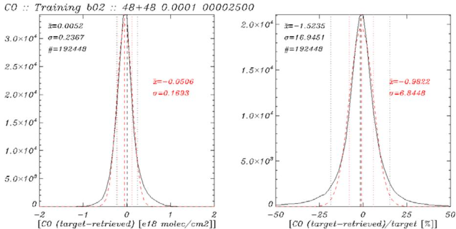
Figure 7 : CO absolute (left) and relative (right) training errors. The overall statistics are displayed in black while the most fitting Gaussian distributions and associated numbers are shown in red. Below, the same statistics without the 7% faintest columns ( $CO < 0.7$  molec/cm<sup>2</sup>).
