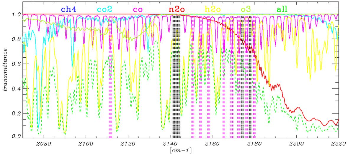
Figure 4 : Modified channel selection for PPFv5.0. Pink and black vertical dash-lines respectively show the absorption and baseline channels involved in the ANN CO retrieval. The various transmittances were computed for a tropical case.
