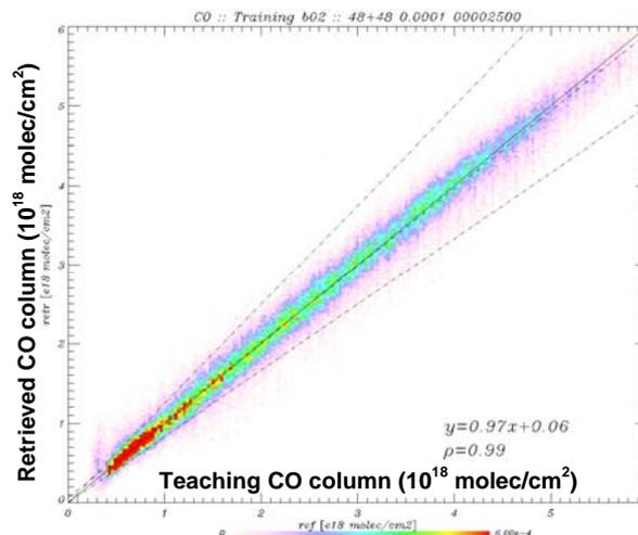
Figure 5 : Linear fit of the retrieved CO total columns to their associated target after training with noisy inputs. Dash-dot lines are the  $\pm 20\%$  showing EURD thresholds.
