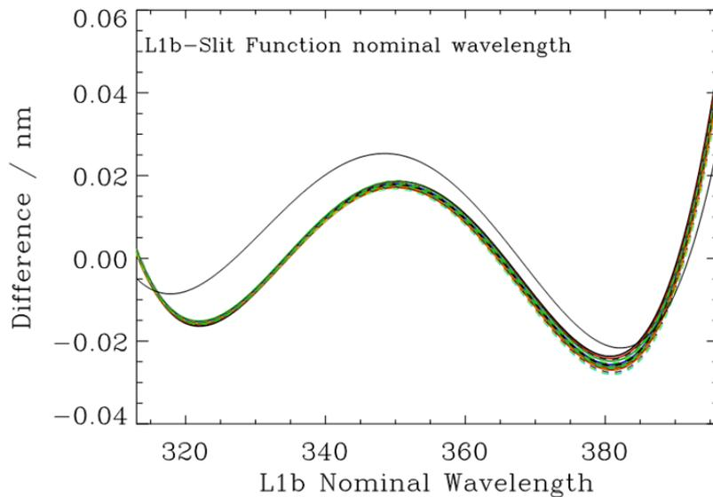
**Figure 1:** The coloured lines show the difference between the GOME2 level 1b nominal pixel wavelengths and those that are obtained by fitting a high resolution solar reference spectrum, convolved with the GOME-2 slit-functions, to the daily solar calibration measurement. Results are shown here for March 2007-February 2008. The black line shows the difference between the level 1b nominal pixel assignment and the central wavelength of the slit function for that pixel.
