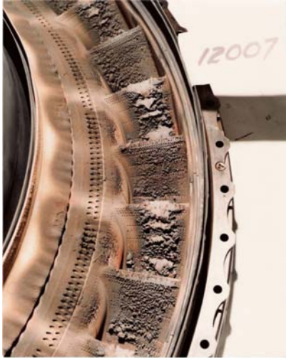
Figure 1: Part of one of the Boeing-747 engines of flight BA-009 after flying through the volcanic ash plume, June 1982. [Photo by captain Eric Moody, British Airways.]
