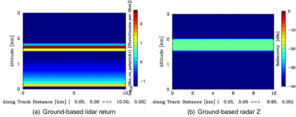
**Figure 2: Ground-based lidar and radar simulation outputs for the single-layer stratocumulus cloud**
