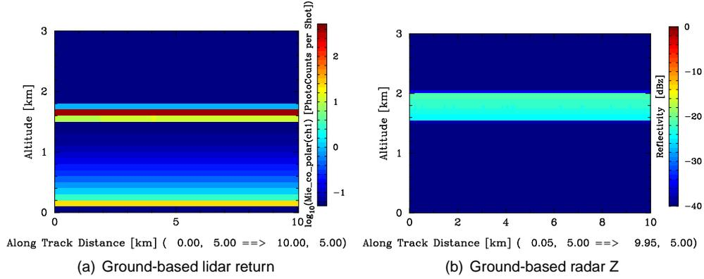
**Figure 3: Ground-based lidar and radar simulation outputs for the single-layer stratocumulus with increasing  $R_{eff}$**
