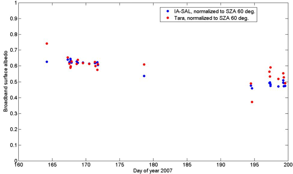
**Figure 4:** Validation results from the Tara drifting ice station. Red circles indicate Tara measurements, blue circles indicate IA-SAL retrievals. All data is normalized to SZA 60 degrees using the algorithm (3).
