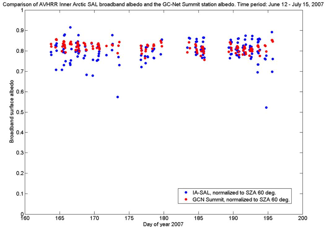
**Figure 3:** Validation results from the GCN Summit station. Red circles indicate GCN measurements, blue circles indicate IA-SAL retrievals. All data is normalized to SZA 60 degrees using the algorithm (3).
