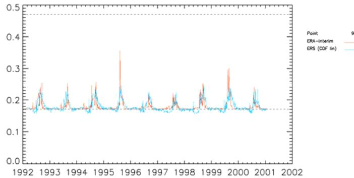
Figure 5 gives an example for the same point as shown above. The systematic bias is reduced by applying Formula 3 and the time series follow a similar temporal pattern. A fact worth noting is that because of the matching technique the lowest values can drop below the wilting point.
