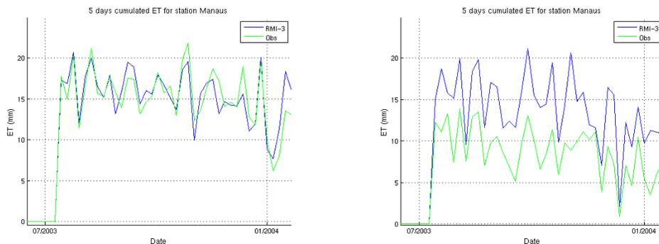
Finally, differences can occur because of differences in meteorological forcing data (Figure 4). Huge differences can exist between observed precipitation data and values extracted from the ECMWF ERA-Interim database. Indeed, for tropical forest station Manaus, ECMWF rains are less intense but more frequent than the observed estimates used as forcing, resulting in doubled cumulated rains that degrade the modelled ET values compared to observations.
