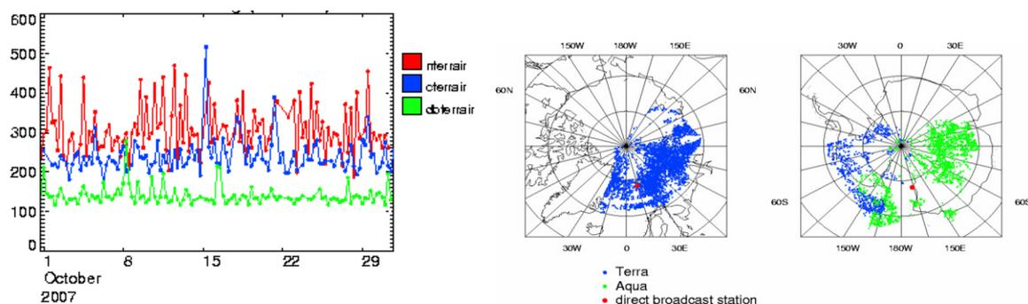
**Figure 4: (left) Mean time lag in minutes between observation time and receipt time for the NESDIS Terra IR winds (red), CIMSS Terra IR winds (blue) and direct broadcast Terra IR winds (green). (right) Data coverage plots showing the coverage of the direct broadcast MODIS winds from Tromsø (receiving station in Svalbard) and McMurdo Station for 0900-1500 UTC on the 7 November 2006.**
