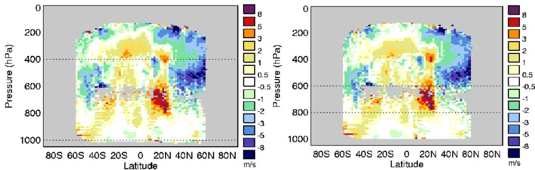
**Figure 3: Zonal O-B speed bias plots comparing Meteosat-9 IR 10.8 AMVs to the Met Office model background (left) and ECMWF model background (right) for December 2008.**
