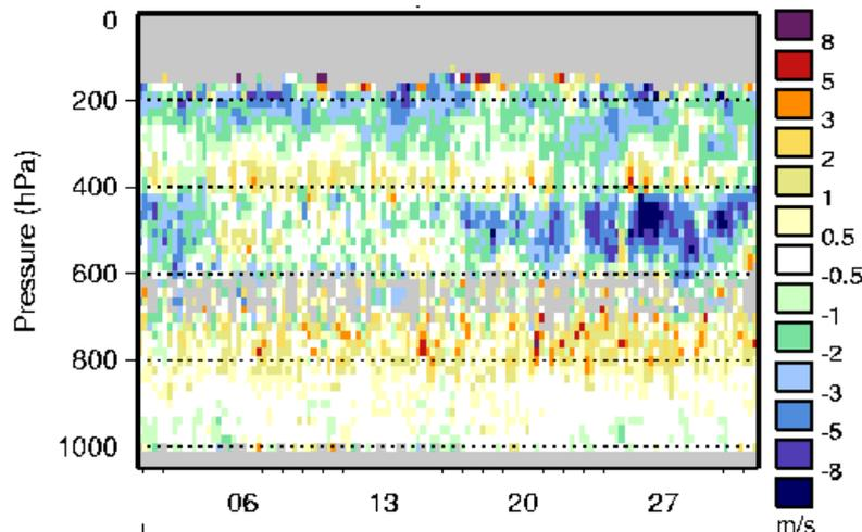
Figure 11: Hovmoeller O-B speed bias plot for Meteosat-9 IR 10.8 NH winds compared with the Met Office model background for October 2008.
