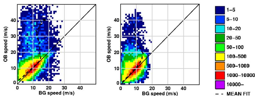
Figure 6: Density plots of observed wind speed against the Met Office model background wind speed for low level winds in the tropics in August 2007 for (left) Meteosat-7 IR and (right) MTSAT-1R IR.
