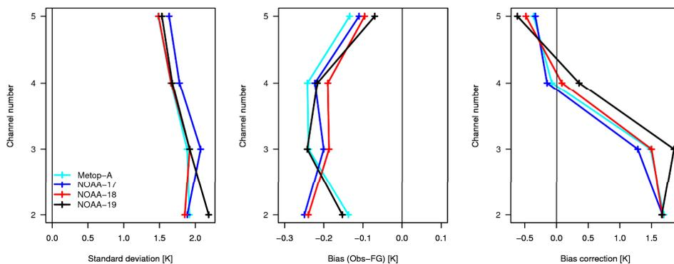
**Figure 2:** As Fig. 1, but for AMSU-B or MHS instruments. NOAA-17 carries an AMSU-B instrument, whereas all other satellites have a MHS instrument. NOAA-19 MHS statistics are based on passively monitored data after quality control, whereas for the other instruments statistics are based on used data or passive data used for quality control.
