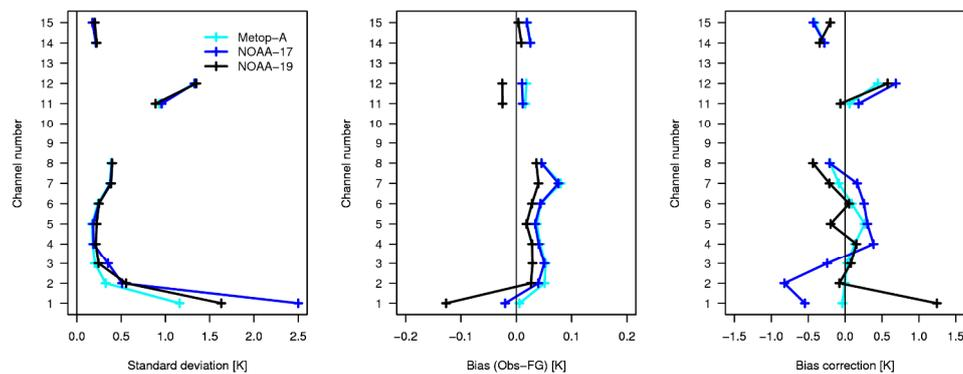
**Figure 3:** As Fig. 1, but for the HIRS instruments. For NOAA-19, statistics are based on passively monitored data after quality control, whereas for the other instruments statistics are based on used data or data used in the quality control.
