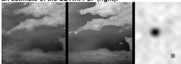
**Figure 13: The 12.0µm SEVIRI image at the left was deconvolved with the model background (centre) to give an estimate of the SEVIRI PSF (right).**
