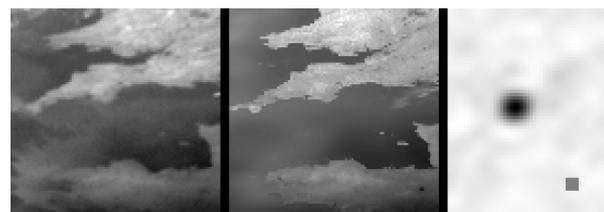
**Figure 12: The 10.8µm SEVIRI image at the left was deconvolved with the model background (centre) to give an estimate of the SEVIRI PSF (right).**
