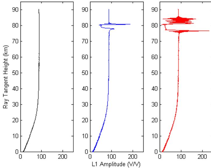
**Figure 6: Simulated amplitudes corresponding to different scintillation conditions. Left panel: no scintillation activity. Medium panel: moderate scintillation activity. Right panel: strong scintillation activity. X-axis: normalized simulated amplitude at LEO (V/V). Y-axis: Ray Tangent Height (Km).**
