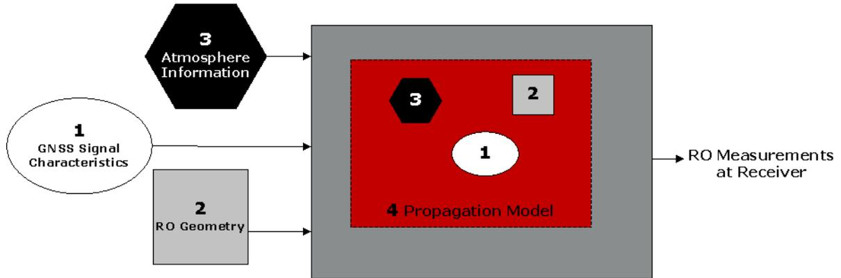
Figure 2: High-level diagram of the RO simulator
