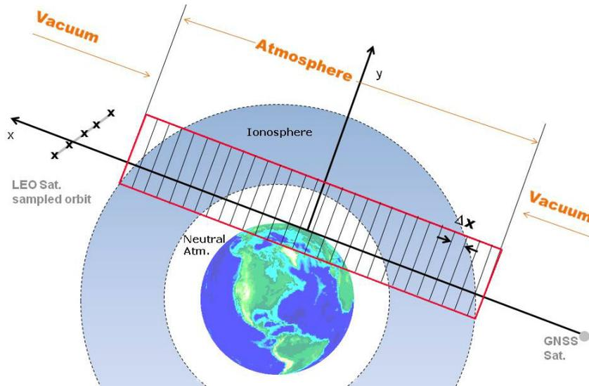
Figure 3: Schematic view of the RO geometry
