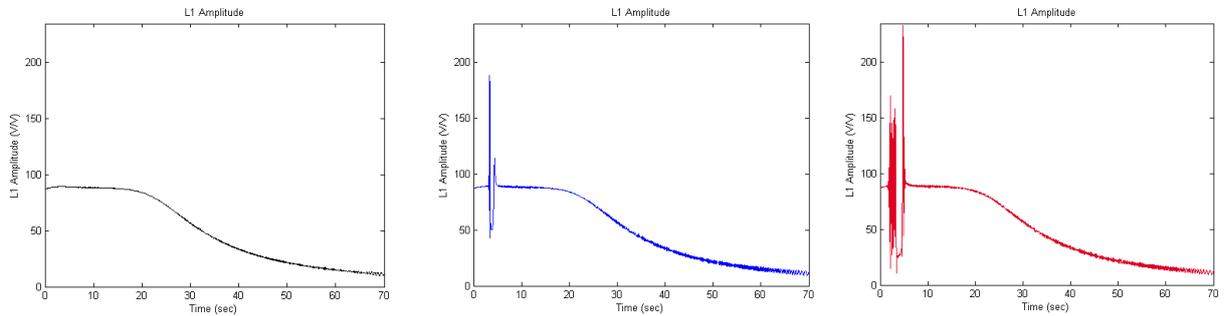
**Figure 5: Simulated amplitudes corresponding to different scintillation conditions. Left panel: no scintillation activity. Medium panel: moderate scintillation activity. Right panel: strong scintillation activity. X-axis: seconds since the start of the occultation event. Y-axis: normalized simulated amplitude at LEO (V/V).**
