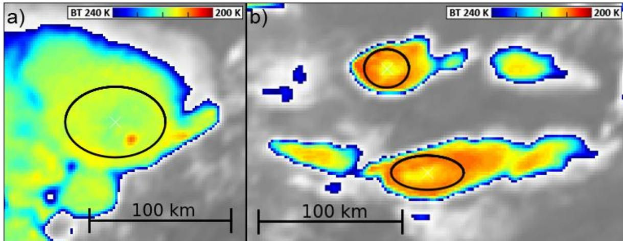
**Figure 2:** Examples of ellipses fitted by the automatic procedure for a) cold-ring-shaped storm with cold overshooting top inside the CWS on 5 July 2012 at 13:25 UTC above Germany; b) two relatively small cold-ring-shaped storms on 11 May 2009 at 16:35 UTC above Austria. For time evolution of parameters of these two ellipses see Fig. 5 and 6.
