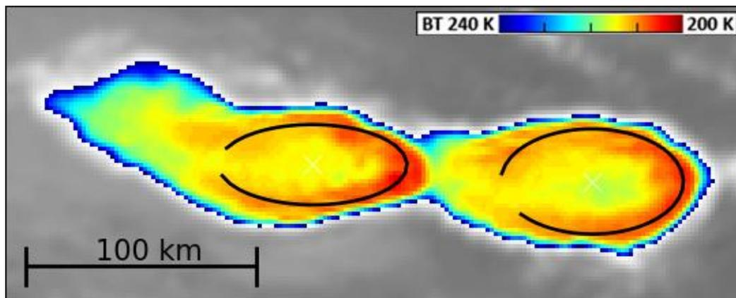
**Figure 3:** Example of parts of ellipses fitted by the automatic procedure illustrating the suitability of the algorithm also for cold-U/V storms. Shown on storms on 31 May 2008 at 13:45 UTC above Germany. For time evolution of parameters of these ellipses see Fig. 4.
