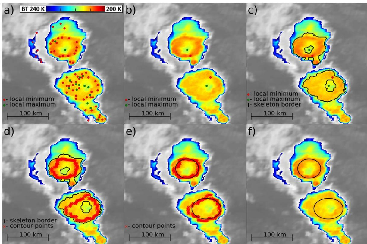
**Figure 1:** Illustration of individual steps of automatic procedure for fitting of cold feature by ellipse showed on storms above the Czech Republic and Austria on 25 June 2006 13:45 UTC. a) detection of local minima and maxima; b) couplet detection; c) detection of skeleton; d) detection of contour points (BT trough); e-f) fitting of contour points by ellipse. For simplicity, steps b-f) are shown only for a single couplet for each feature.
