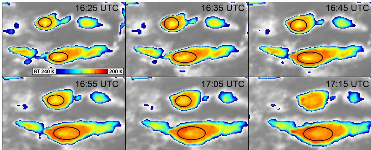
**Figure 6:** Example of time evolution of fitted ellipses shown on storms on 11 May 2009 above Austria. For time evolution of parameters of these ellipses see Fig. 5. In the last frame (17:15 UTC) the north ellipse is not detected any more as the temperature difference between the embedded warm area and cold part of the feature is too small.
