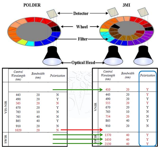
The 3MI spectral bands are shown in table for comparison this table contains also the POLDER / PARASOL spectral bands. Red color is used to indicate the main differences. Channels 354 nm and 388 nm, originally considered for 3MI, have been replaced by the channel at 410 nm, in order to reduce risk and maintain affordability of the instrument.
