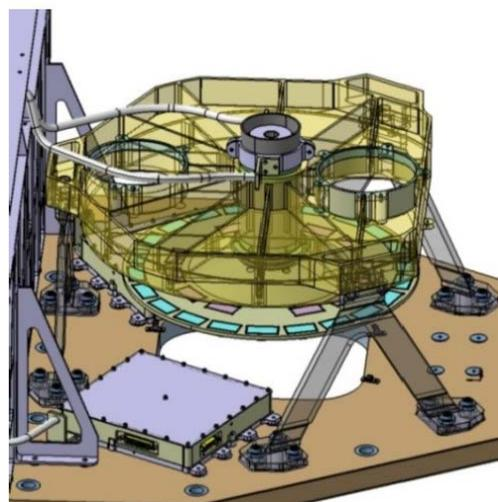
***Filter wheel and its mechanism***
