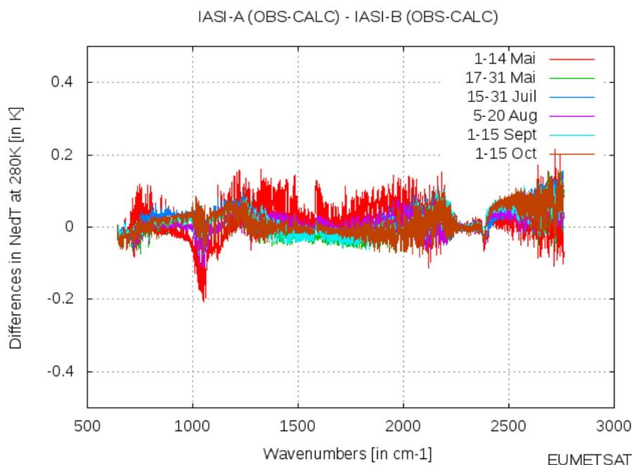
**Figure 2: Differences between IASI-A (OBS-CALC) and IASI-B (OBS-CALC) in NedT at 280K for different periods of time since the end of IASI-B commissioning.**
