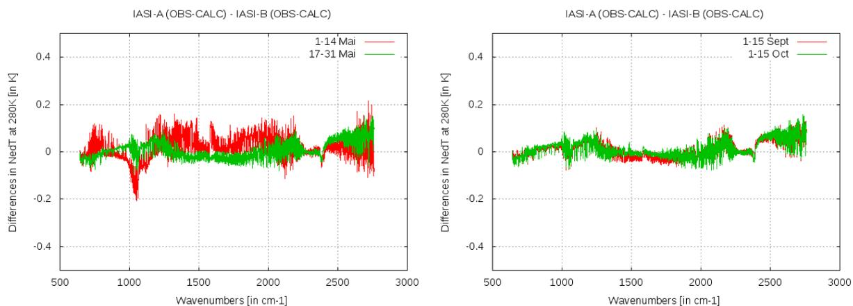
**Figure 3: On-ground updates for the IASI level 1 processing for both IASI, in May on the left and in September on the right. Before the update is shown in red, and after in green.**
