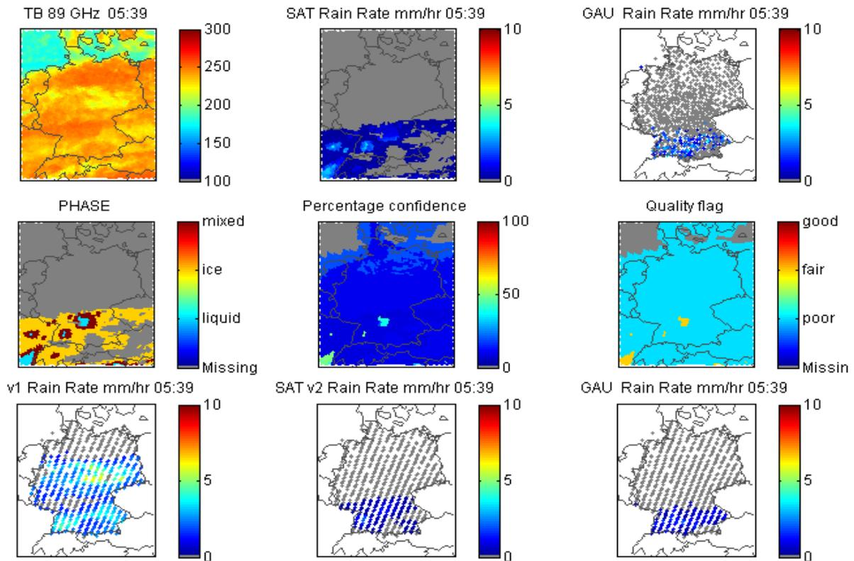
**Figure 2:** Same as Fig. 1 but for CDRD and for winter front case study GE03 06/12/2010 05:39 UTC. In the last row results from the old version (H01 ver. 1.4) and the new version (H01 ver. 1.7) are compared to the gauges.
