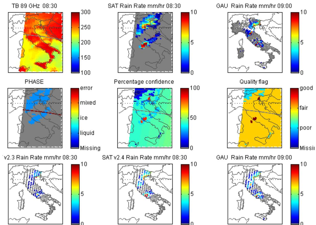
**Figure 1:** Results for PNPR and flash flood case study IT1 20/10/2011 08:30 UTC. Top row from left to right: TB at 89 GHz, PNPR (H02 ver. 2.4) surface precipitation rate; hourly precipitation from gauges. Second row: Phase flag, PCI, quality index. Bottom row: precipitation rate from old version (H02 ver. 2.3) and new version (H02 ver. 2.4), hourly precipitation from gauges (spatially averaged).
