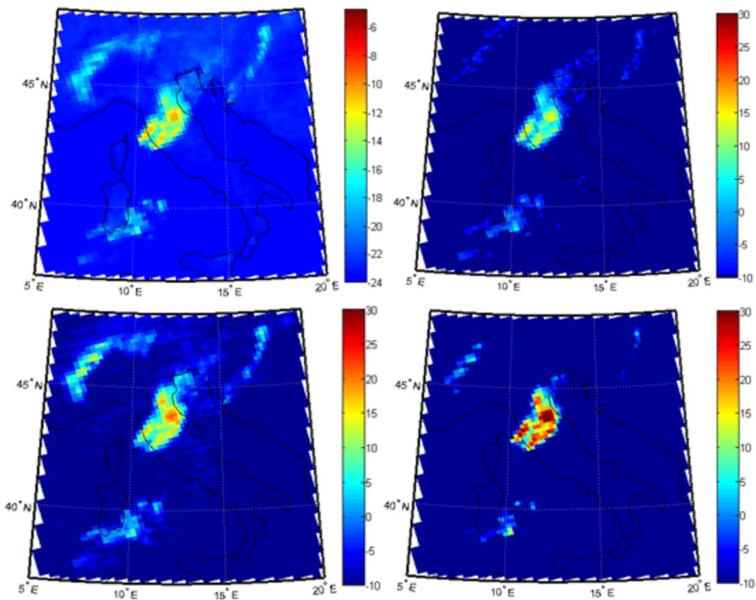
**Figure 3:** Grosseto flood (11 and 12 November 2012). The top panels show (from left to right) the CCA (obtained using the TBs of 50, 89 and 150 GHz channels, for the selected overpass of NOAA-18 AMSU-A/MHS at 13:25 UTC on 12 November, 2012) and the  $\Delta_{17}$  difference. The bottom panels show the  $\Delta_{37}$  (left) and  $\Delta_{13}$  (right) differences.
