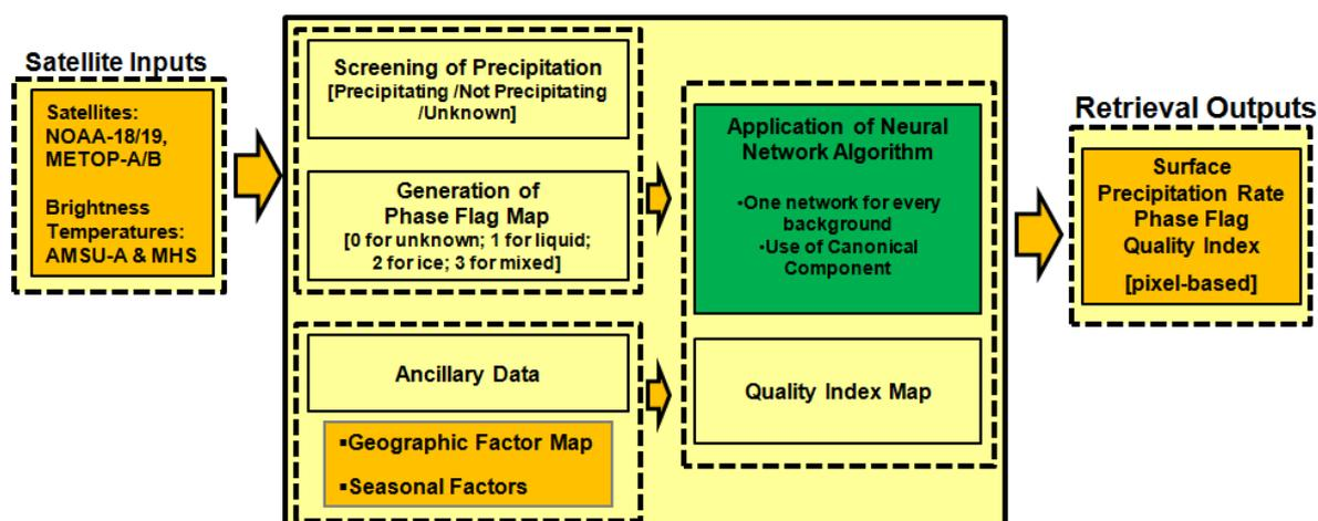
Figure 2: Block diagram of the PNPR algorithm
