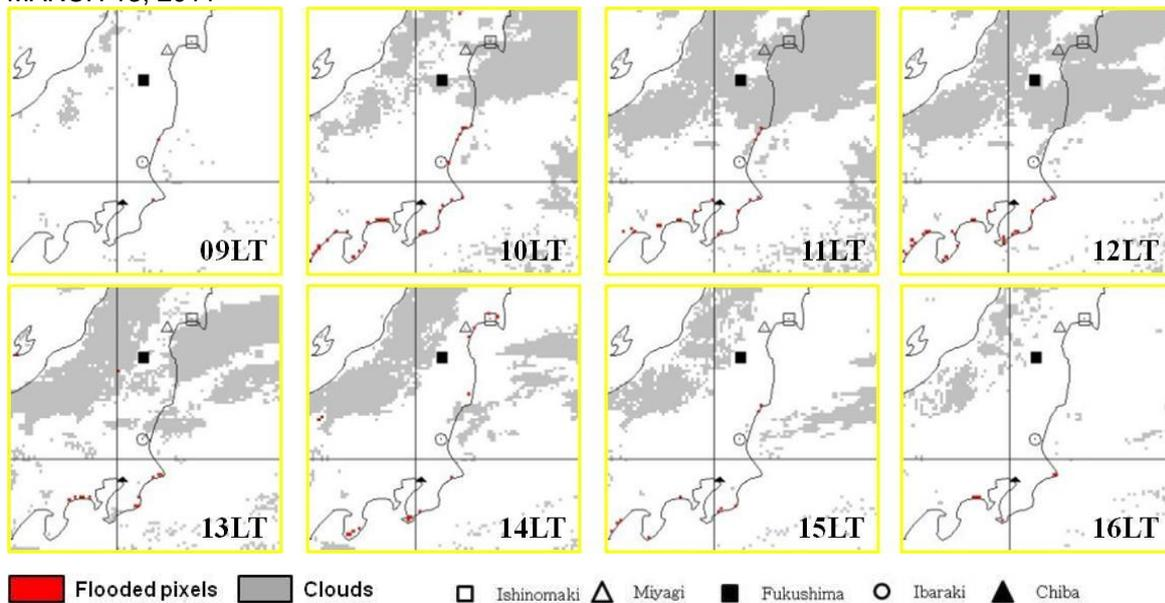
**Figure 6.** Detection of flooded pixels (in red) along the Japanese coasts for March 12 (on the top) and 13 (on the bottom) using Eq. 3.
