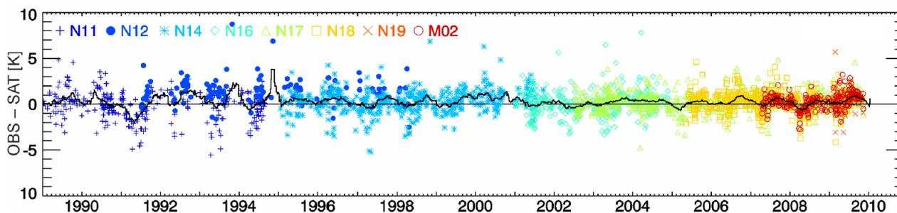
**Figure 2:** Time series of the difference in LST between in-situ (OBS) and satellite-based LST at Bregener Hafen, Lake Constance (Riffler and Wunderle, *in prep.*). Symbols indicate the satellite used for LST retrieval (NOAA: N11-N19; Metop-A: M02).
