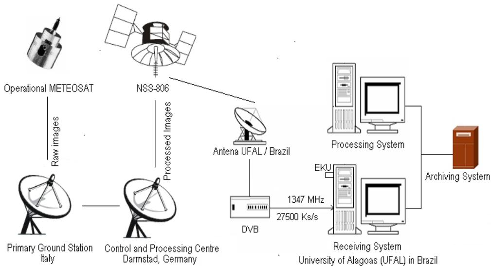
**Figure 3: Overview of the broadcasting ground reception and processing system at the University of Alagoas (UFAL) in Brazil.**
