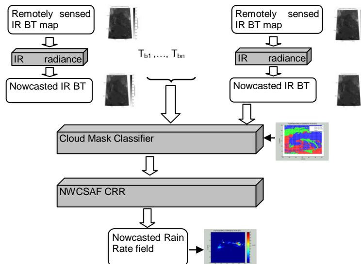
**Figure 1:** The MeteoCAST logical layout: the flow goes from the MSG images acquisition to the rain rate estimation.
