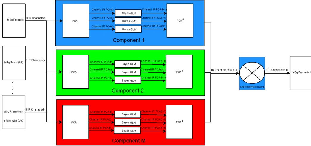
**Figure 2: The nowcasting architecture. The frames in input are broadcasted to each ensemble's components and the output of each component is mixed to give the ensemble's output.**
