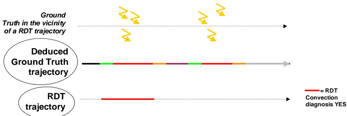
Figure 4: Validation outline. The electrical-trajectory (ground truth trajectory) is built with the strokes in the vicinity of a RDT trajectory (upper part of the figure). Some sections are then defined for deduced ground truth trajectory (middle part). The RDT convection diagnosis (lower part) is compared to electrical observed ground truth.
