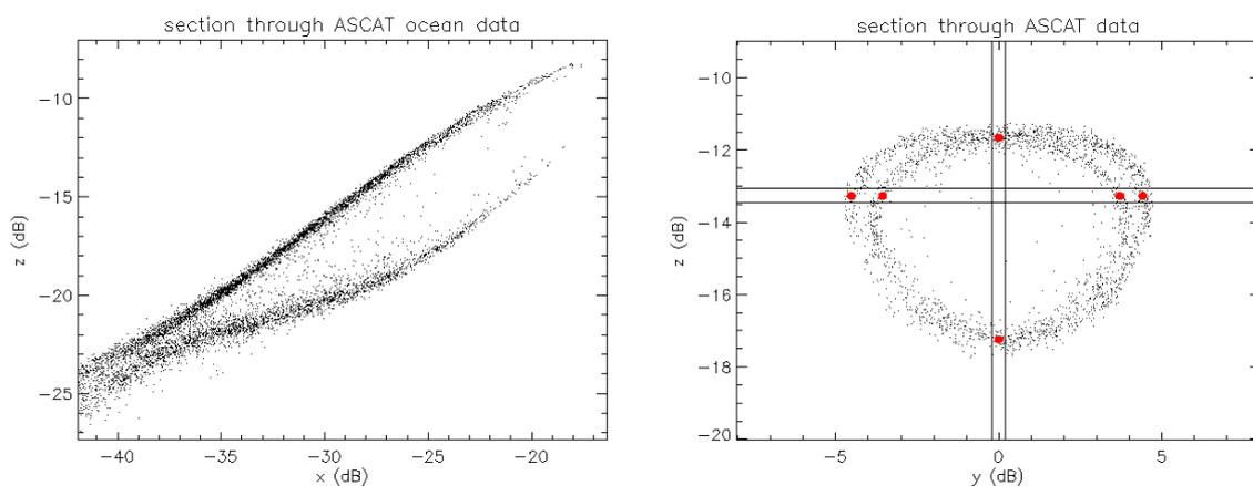
**Figure 9: Example of sections through a month of ASCAT-B data from the open ocean with the position of maximum data density in two slices marked in red. These sections vary with incident angle.**
