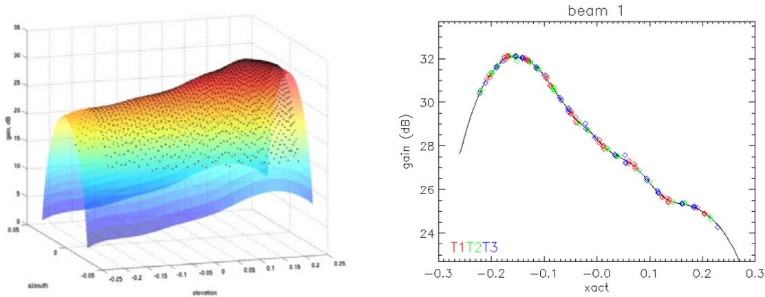
**Figure 5: (a) Example gain pattern as a function of antenna elevation and azimuth angles and (b) a section through LEFT MID beam gain pattern as a function of elevation angle.**
