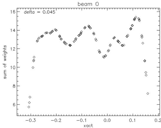
Figure 7: Sum of the weights used to fit the low order polynomial in the kernel smoothing for the LEFT FORE beam.
