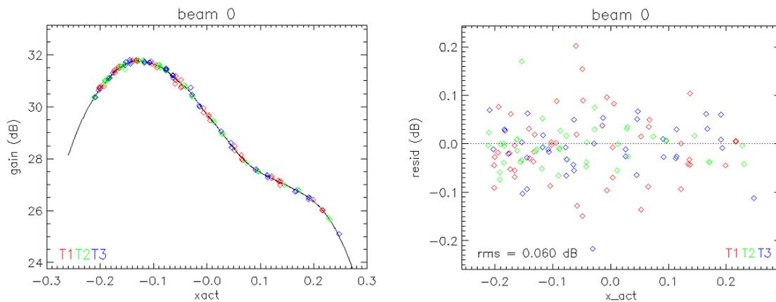
**Figure 6: (a) Transponder data with the fitted gain model and (b) the residual between data and model, for the LEFT FORE beam**
