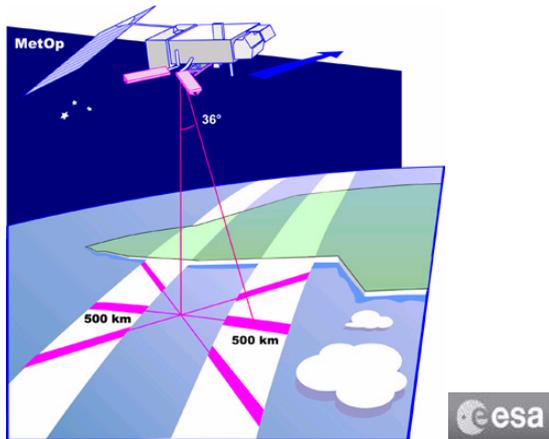
**Figure 1: Schematic showing the viewing geometry of the ASCAT.**
