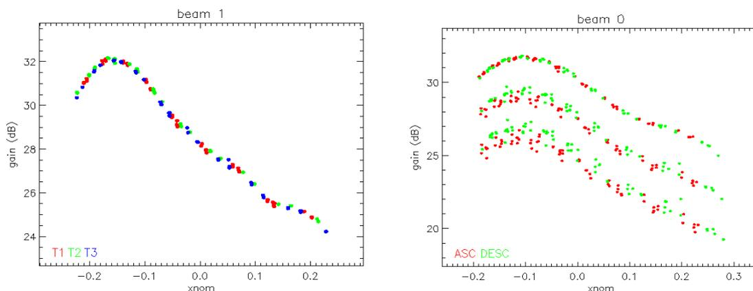
Figure 4: (a) transponder data LEFT MID beam, showing minor distortion and (b) transponder data in LEFT FORE beam at three different azimuth angles, showing differences between ascending and descending passes.
