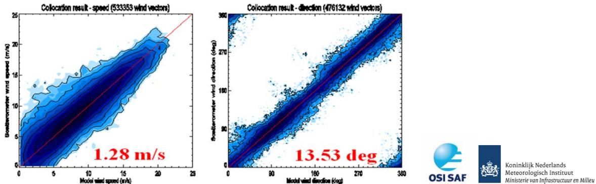
Figure 11: Difference in wind speed and direction between wind vectors derived from ASCAT-B data and ECMWF NWP output. Plots courtesy of KNMI (OSI-SAF).
