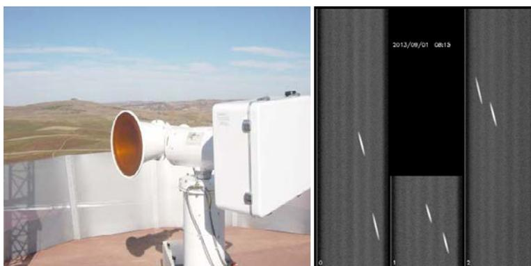
Figure 3: (a) Transponder on site in Turkey and (b) transponder signals in ASCAT calibration data.
