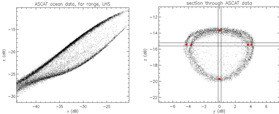
**Figure 5: (left) Section along the ASCAT-A NRCS cone for a mid-swath location; (right) Section across the ASCAT-A cone for a mid-swath location. Red dots represent the location of highest density data in the vertical and horizontal slices shown in the figure. The data represented in these plots corresponds to the global oceans during a 29 day orbit repeat cycle.**
