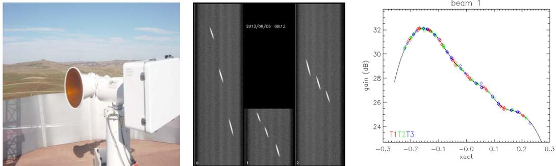
Figure 1: (left) Tranponder on site in Turkey; (centre) Image of raw transponder signams captured by ASCAT-A; (right) Estimation of gain from the transponders with the fitted gain model for the LEFT MID beam of ASCAT-A
