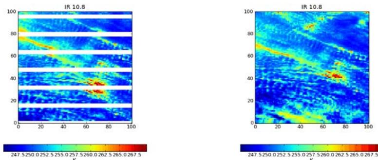
**Figure 2:** Raw 11micron brightness temperature image (left); after adjacency algorithm is applied (right)
