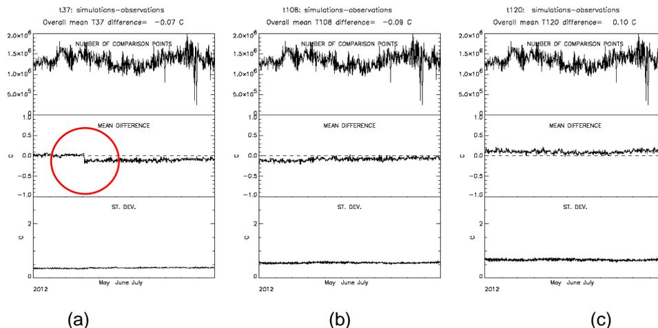
**Figure 3:** Mean daily differences and standard deviation between simulated and observed METOP/AVHRR brightness temperatures, from December 1<sup>st</sup> 2011 till December 1<sup>st</sup> 2012, a) 3.7; b) 10.8 and c) 12.0  $\mu\text{m}$ .
