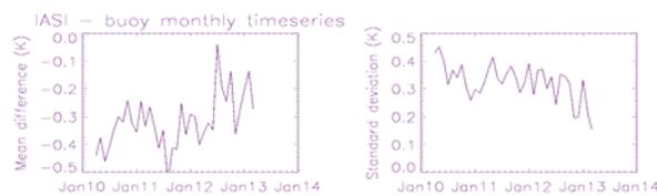
Figure 7. Monthly time-series of IASI minus buoy mean differences and standard deviations.
