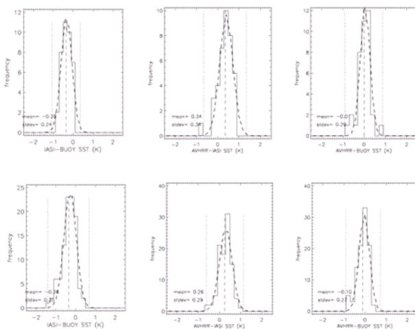
Figure 8. Histograms of IASI minus buoy, AVHRR minus IASI, and AVHRR minus buoy differences, for Metop-B (top) and Metop-A (bottom) over the period July 2012 to July 2013.
