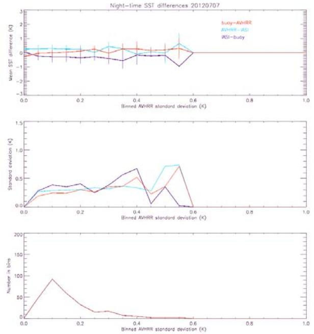
Figure 4. IASI minus buoy SST versus standard deviation of 21x21 AVHRR observations over the period July 2012 to July 2013.
