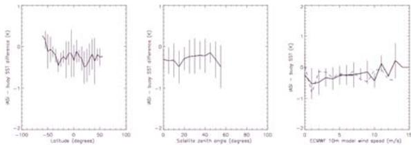
Figure 2. Binned plots of IASI minus buoy differences versus latitude, satellite zenith angle and ECMWF wind-speed over the period July 2012 to July 2013.
