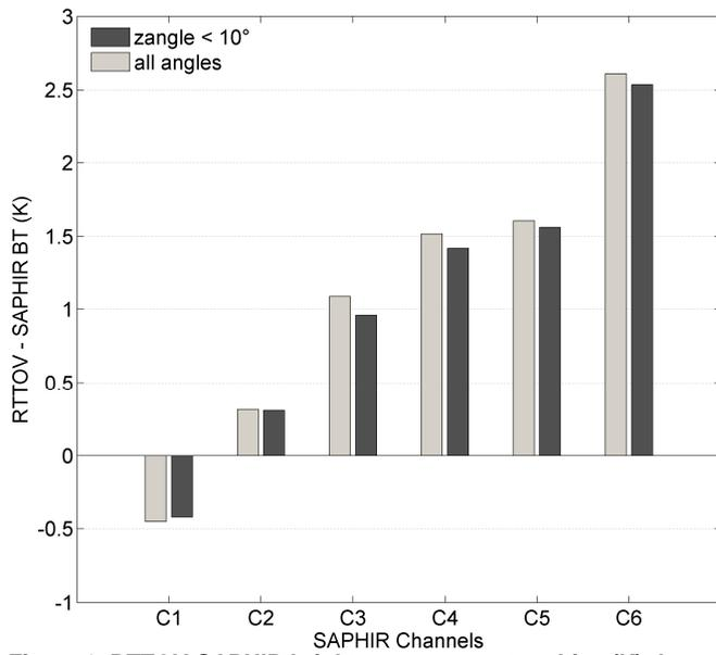
**Figure 3: RTTOV-SAPHIR brightness temperature bias (K) dependence to zenith angle.**
