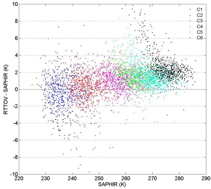
**Figure 2: RTTOV-SAPHIR brightness temperature bias (K) dependence to observed SAPHIR brightness temperatures.**
