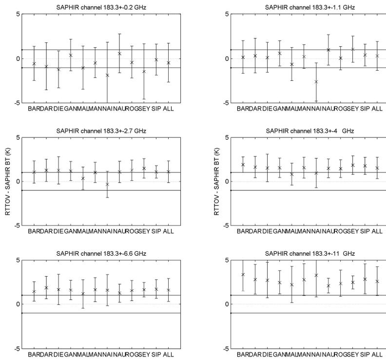
**Figure 4: RTTOV-SAPHIR brightness temperature bias (K) for each saphir channel and each Cindy - Dynamo radisonde launch site used in the database. Errorbars depict standard deviations (K) restricted to a single site.**
