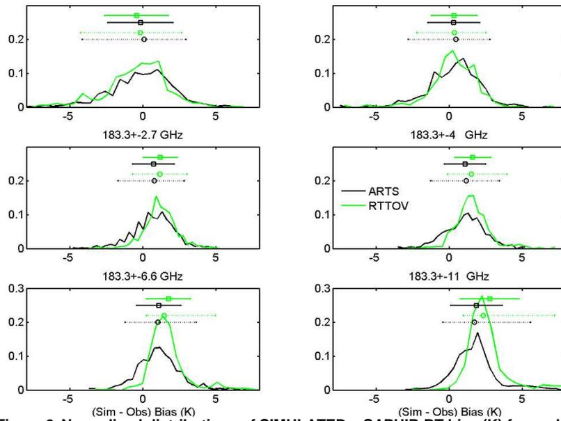
**Figure 6: Normalised distributions of SIMULATED – SAPHIR BT bias (K) for each SAPHIR channel, RTTOV (green lines) and ARTS (black lines). Square marks and plain lines show mean and standard deviation. Circle marks and dotted lines show median, 5<sup>th</sup> and 95<sup>th</sup> centiles.**
