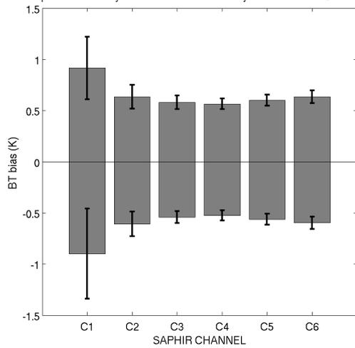
**Figure 5: Sensitivity of RTTOV radiative transfer model to a perturbation of the input RH profile according to the extreme values of the calibration uncertainty for daytime observations. Grey bars show the mean output BT change (K) with regards to reference simulation, black errorbars show the standard deviation (of change in output BT (K) with regards to reference simulations).**
