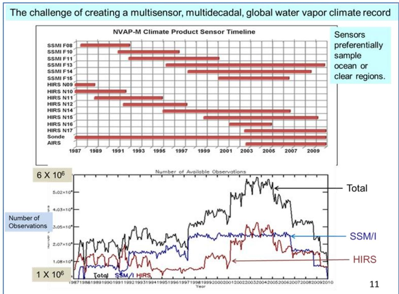
Figure 1: NVAP-M sensor timeline, and time series of number of total, SSM / I and HIRS observations.
