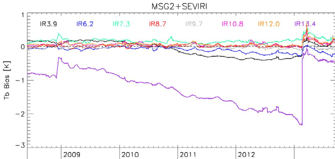
**Figure 1:** Time series plot showing relative bias of IR channels of Meteosat-9/SEVIRI (MSG2) wrt Metop-A/IASI, expressed as brightness temperature difference for standard radiance scenes (corresponding to a 1976 US Standard Atmosphere with clear sky). Spacecraft decontaminations in Dec 2008 and Feb 2013 introduced step bias changes.
