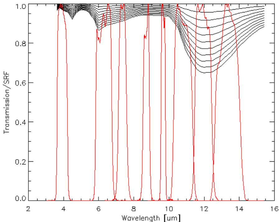
**Figure 4: Transmittance spectra due to absorption by ice layers of different thicknesses (black): 0.1 to 1.0  $\mu\text{m}$  layers (thickest layers have lowest transmittance) and Spectral Response Functions of Meteosat-8 infrared channels (red).**
