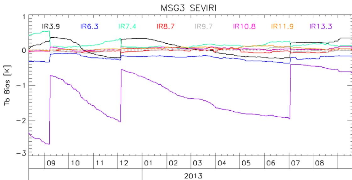
**Figure 2:** As Figure 1, but for Meteosat-10/SEVIRI (MSG3). Decontaminations in September and December 2012 and July 2013 introduced step bias changes.
