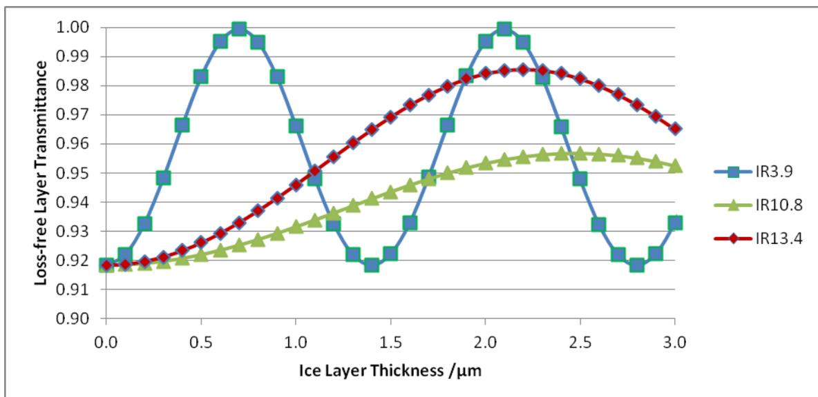
Figure 5: Transmittance through lossless dielectric layer of ice deposited on a planar slab with  $n=1.8$ .
