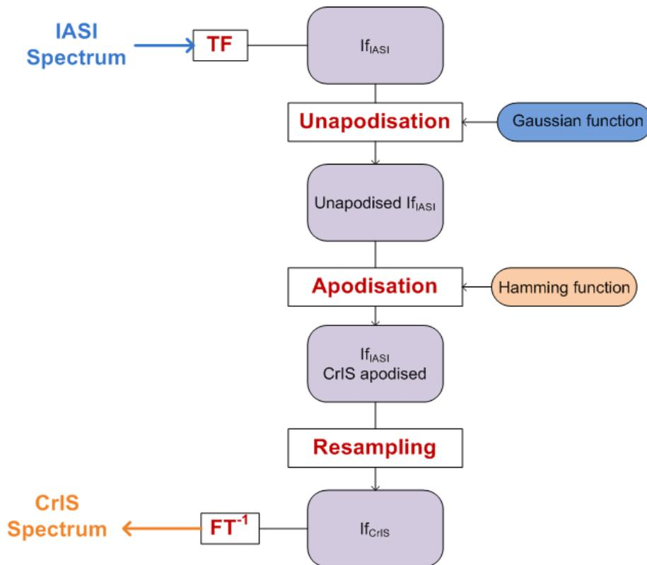
Figure 1: flowchart of the transformation of a IASI spectrum into its CrIS-like equivalent.
