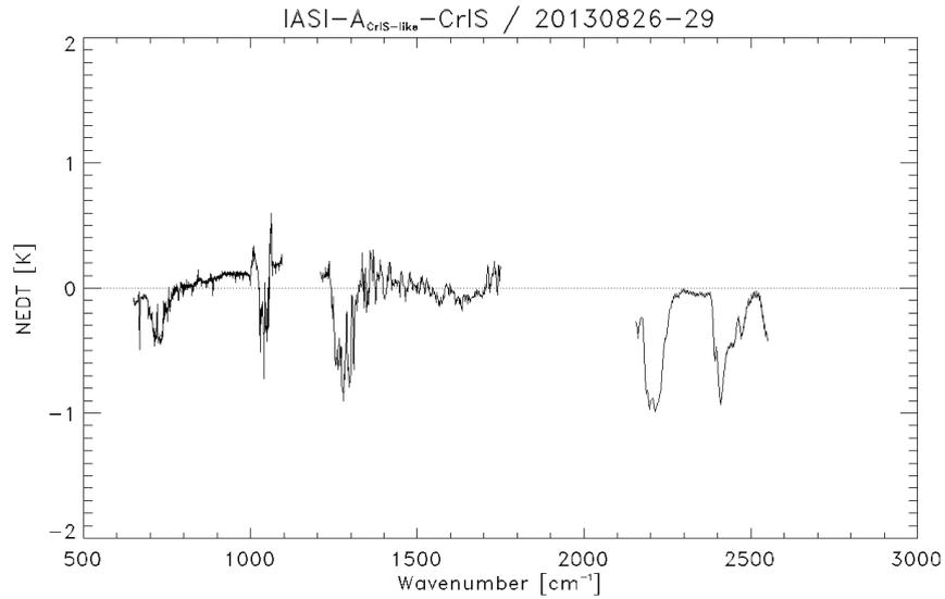
**Figure 7: Spectral difference IASI-A – CrIS computed from the residuals OBS-CALC for both instruments for four days in August 2013.**
