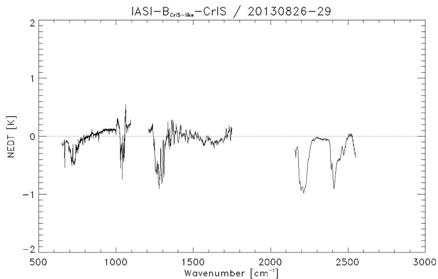
**Figure 8: Spectral difference IASI-B – CrIS computed from the residuals OBS-CALC for both instruments for four days in August 2013.**
