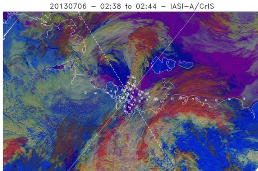
**Figure 2:** geographical distribution of the IASI (+ signs) and CrIS (squares) pixels selected for the comparison during a single SNO event between Metop-A and NPP on 6<sup>th</sup> July 2013 around 02:40. The straight lines are the satellite tracks. The background in an AVHRR image in false colours in which sea appears as deep blue, land as light blue, sea ice as purple and clouds are in white-green-red.
