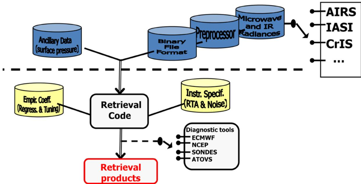
**Figure 1.** Modular retrieval architecture of the NOAA Operational Hyper Spectral Retrieval Algorithm
