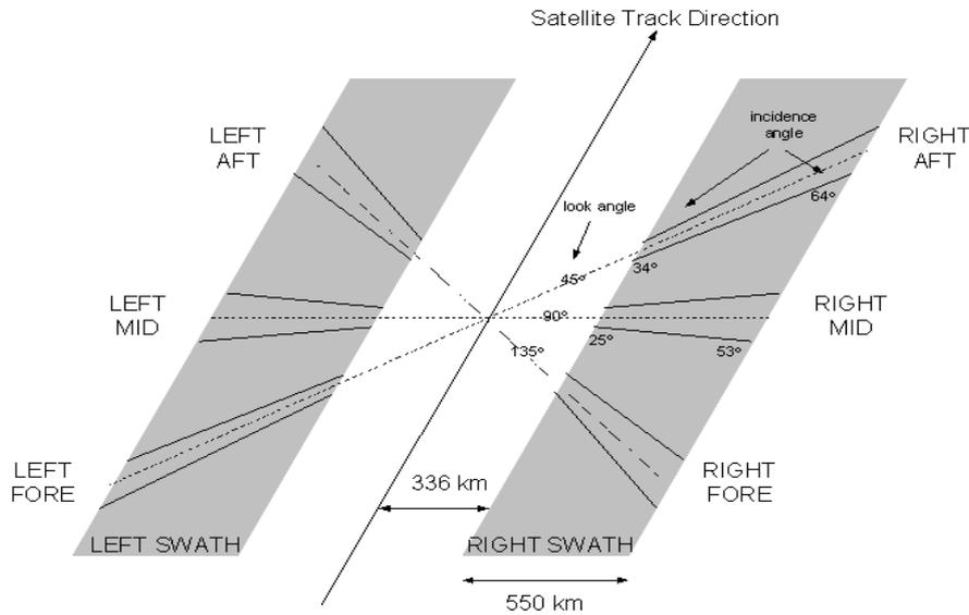
Figure 4: Swath geometry of the ASCAT antennas for a reference orbit height of 822 km.
