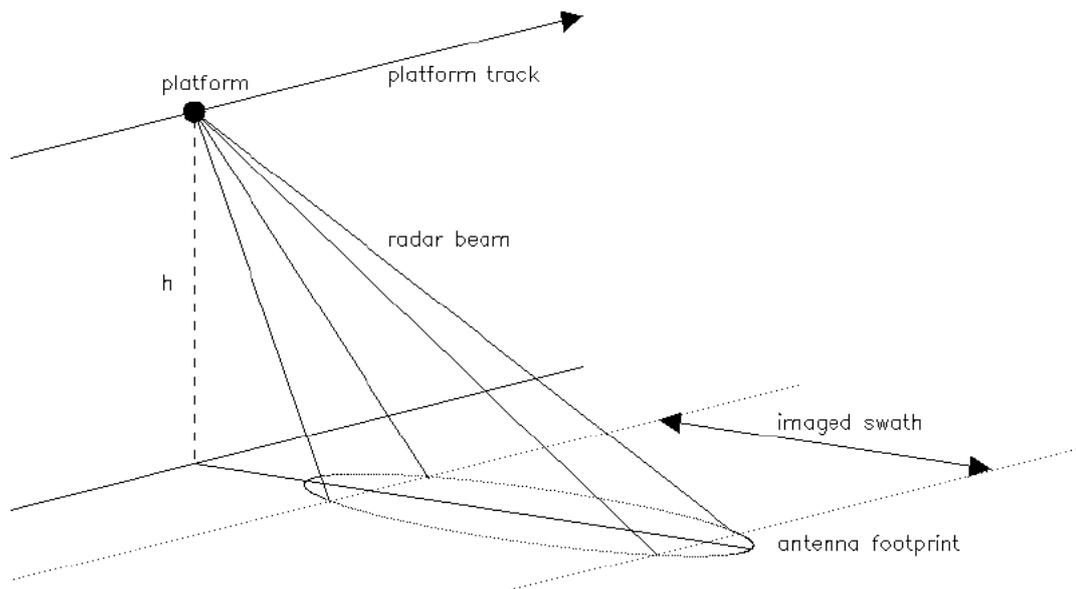
*Figure 3: Basic geometry of a side-looking radar.*
