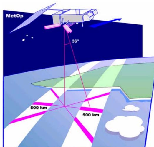
*Figure 1: Viewing geometry of the ASCAT.*
