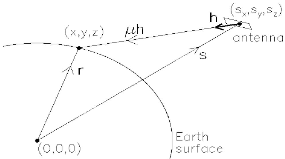
Figure 6: Geometry of an ASCAT antenna viewing the Earth.
