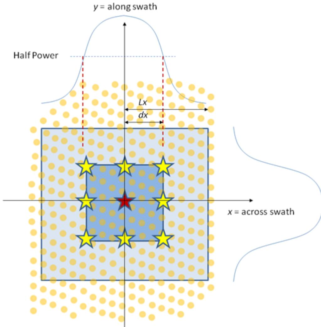
Figure 5: Schematic representation of the ASCAT NRCS re-sampling approach.
