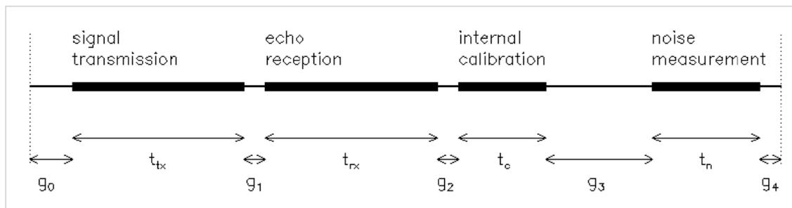
Figure 2: ASCAT transmit/receive timeline.
