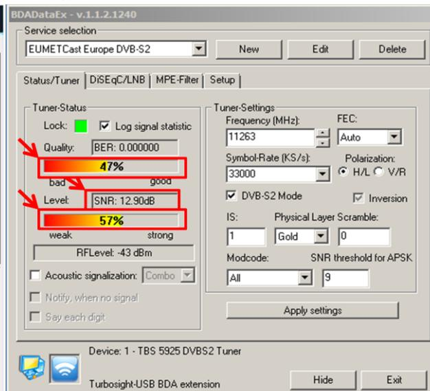
**Figure 3 TBS-5925 Measurement Checking - EUMETCast Europe Ku-Band**
