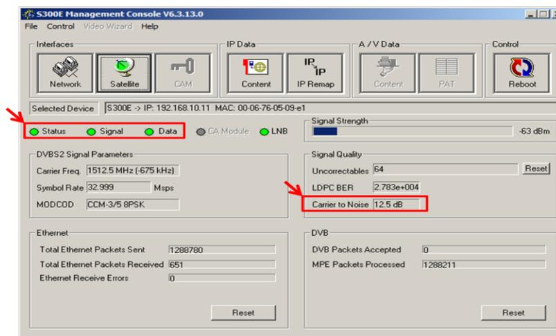
Figure 2 NOVRAS300E Measurement Checking - EUMETCast Europe Ku-Band
