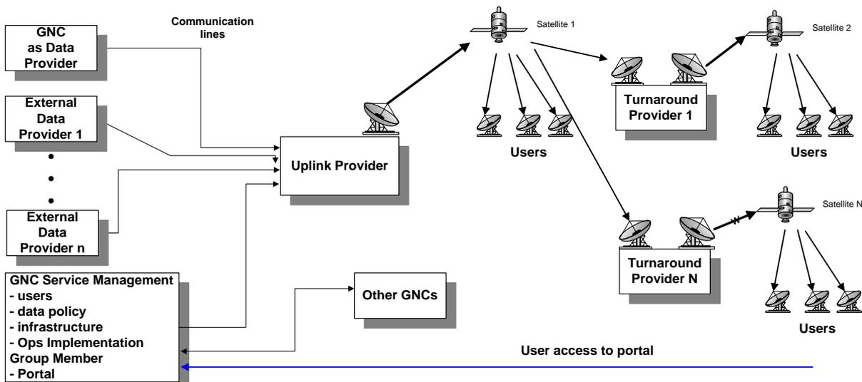
Each GNC would comprise the same components of 1) Data acquisition, 2) Service management, 3) Uplink provider, 4) Turn around providers and 5) User community (figure 4 above) and additionally 5) cooperates with the partner GNCs over communication links.
