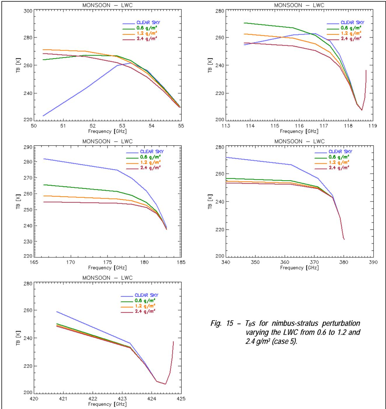
**Fig. 15** -  $T_{BS}$  for nimbus-stratus perturbation varying the LWC from 0.6 to 1.2 and 2.4 g/m<sup>3</sup> (case 5).
