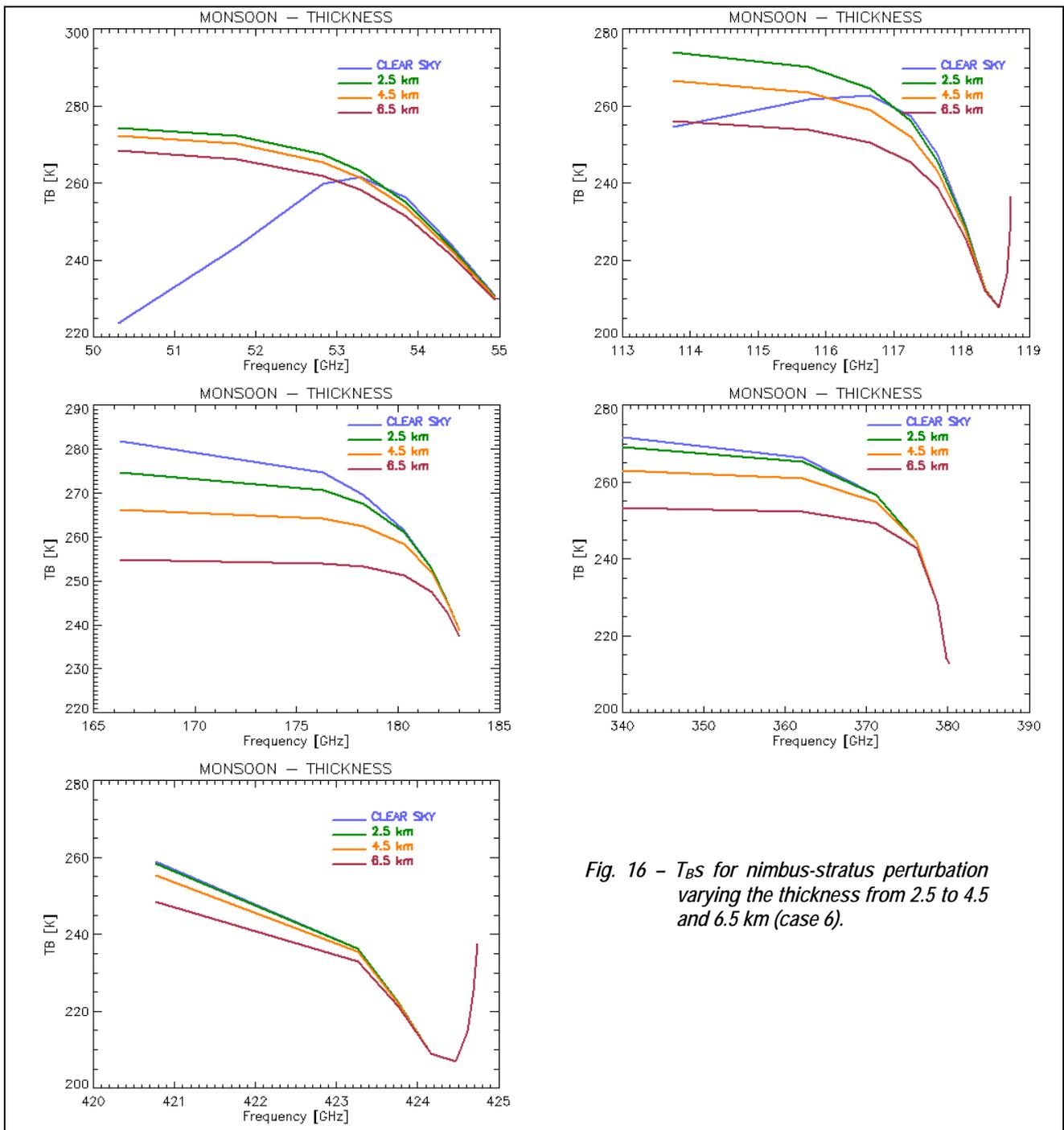
Fig. 16 -  $T_{BS}$  for nimbus-stratus perturbation varying the thickness from 2.5 to 4.5 and 6.5 km (case 6).
