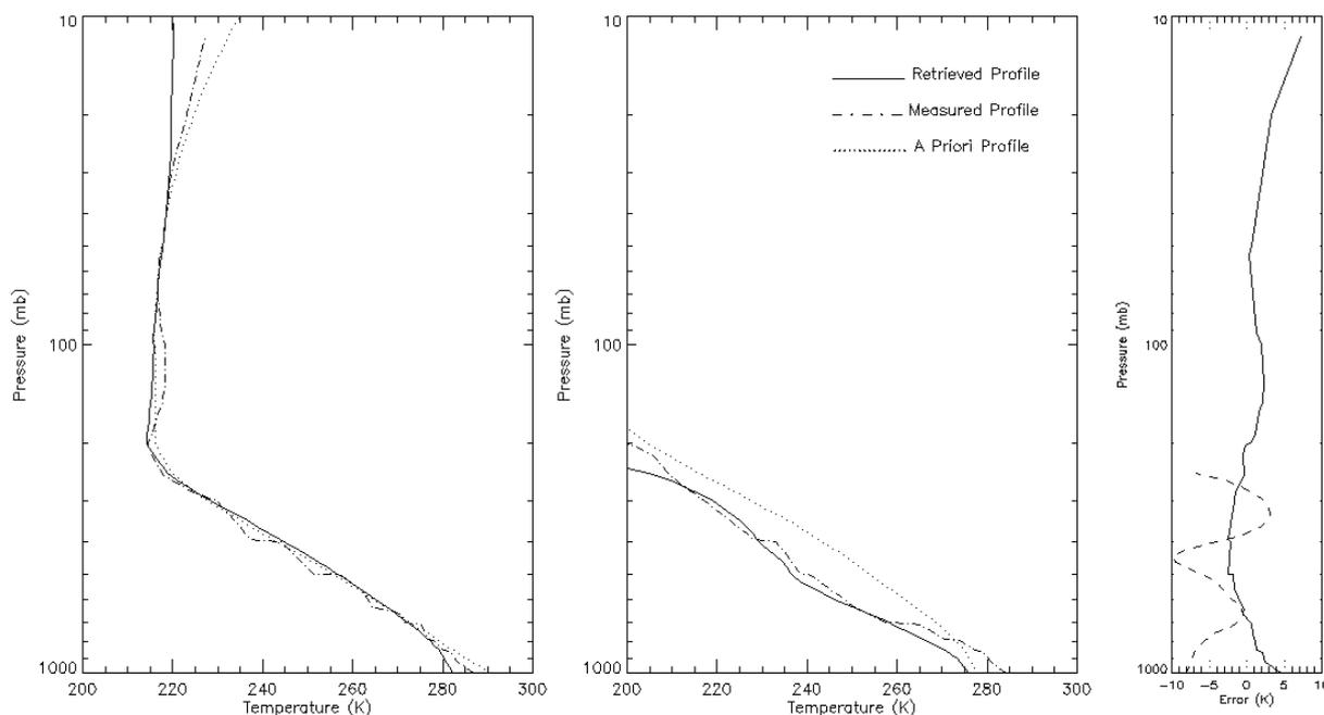
*Fig. 6 – Retrieval versus radiosonde profiles at Milano Linate (Italy), on 15 May 2005 at 00 UTC. In the right panel the retrieval errors are show (temperature solid line, dew-point dashed line).*
