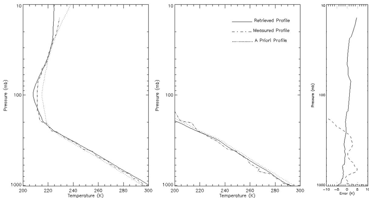
*Fig. 7 – Retrieval versus radiosonde profiles at Pratica di Mare (Italy), on 23 June 2005 at 00 UTC. In the right panel the retrieval errors are show (temperature solid line, dew-point dashed line).*
