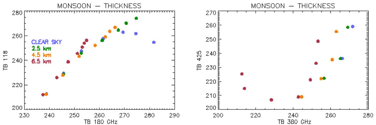
Fig. 22 - Scatterplots between two band association to retrieve water vapour in case 6 (nimbus-stratus with changing thickness). Left: 183 v/s 118 GHz; right: 380 v/s 425 GHz.
