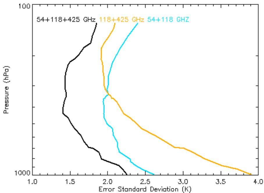
*Fig. 9 – Standard deviation of retrievals from different combinations of the three O<sub>2</sub> bands.*
