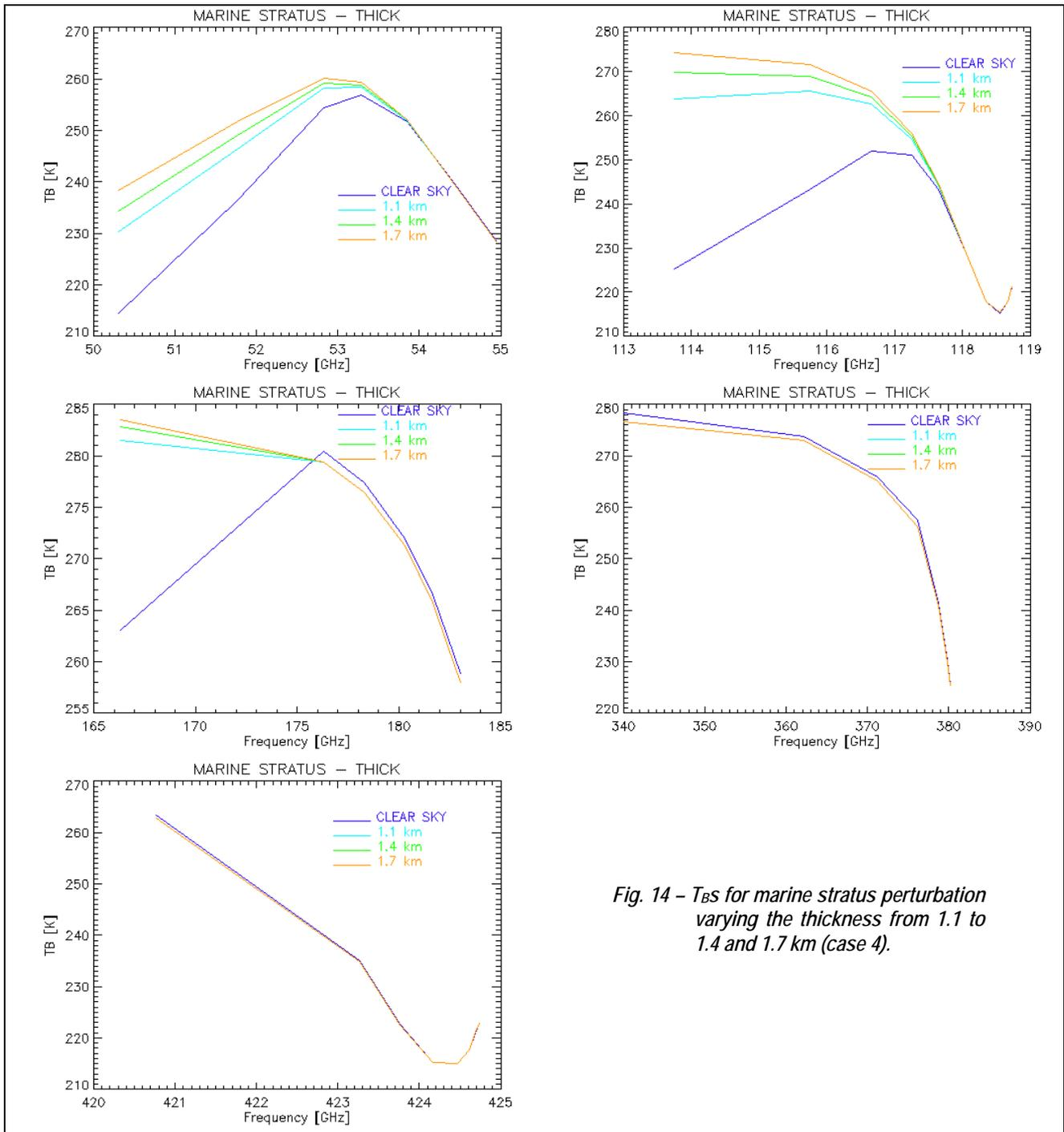
Fig. 14 –  $T_B$ s for marine stratus perturbation varying the thickness from 1.1 to 1.4 and 1.7 km (case 4).
