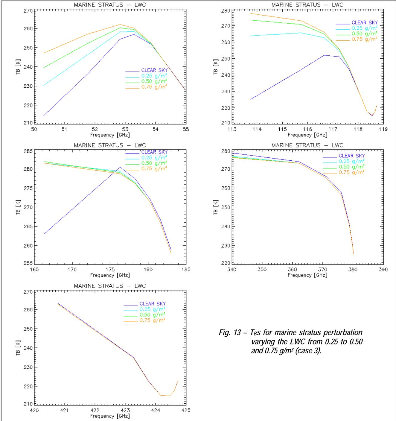
**Fig. 13** –  $T_{BS}$  for marine stratus perturbation varying the LWC from 0.25 to 0.50 and 0.75 g/m<sup>3</sup> (case 3).
