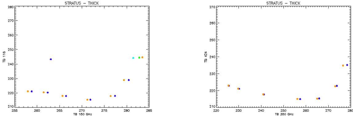
Fig. 20 - Scatterplots between two band association to retrieve water vapour in case 4 (maritime stratus with changing thickness). Left: 183 vs. 118 GHz; Right: 380 vs. 424 GHz.
