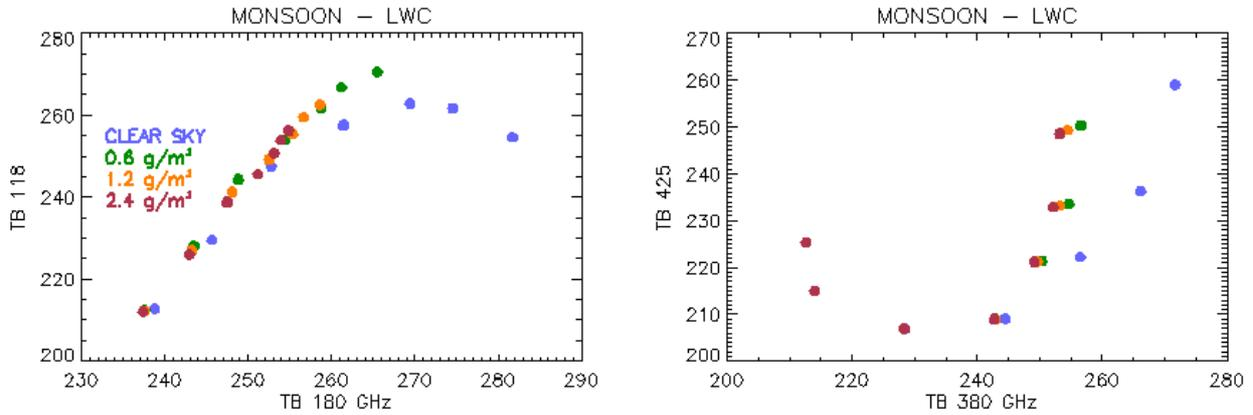
Fig. 21 - Scatterplots between two band association to retrieve water vapour in case 5 (nimbus-stratus with changing LWC). Left: 183 v/s 118 GHz; right: 380 v/s 425 GHz.
