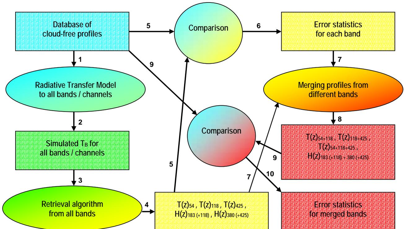
Fig. 3 – Architecture of the study for clear-air temperature-humidity profile characterisation.
