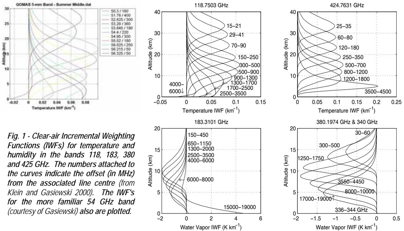
Fig. 1 - Clear-air Incremental Weighting Functions (IWFs) for temperature and humidity in the bands 118, 183, 380 and 425 GHz. The numbers attached to the curves indicate the offset (in MHz) from the associated line centre (from Klein and Gasiewski 2000). The IWF's for the more familiar 54 GHz band (courtesy of Gasiewski) also are plotted.
