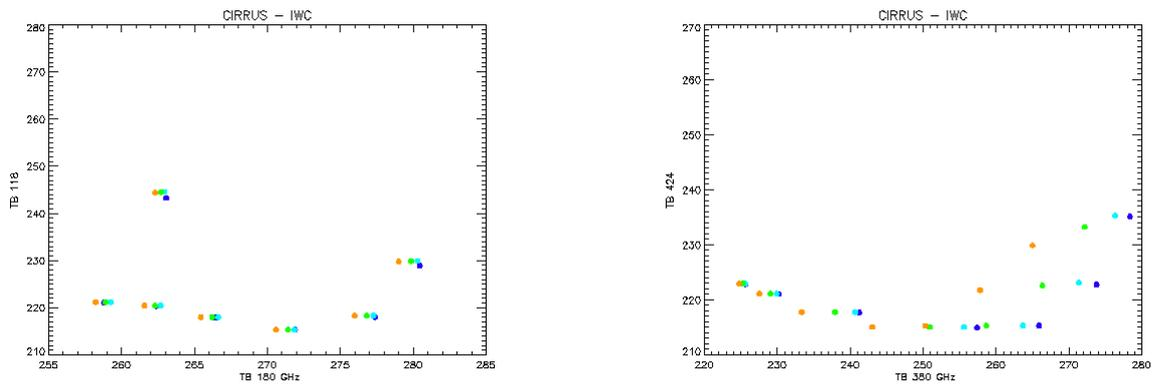
*Fig. 17 – Scatterplots between two band association to retrieve water vapour in case 1 (cirrus with changing IWC). Left: 183 v/s 118 GHz; right: 380 v/s 425 GHz.*
