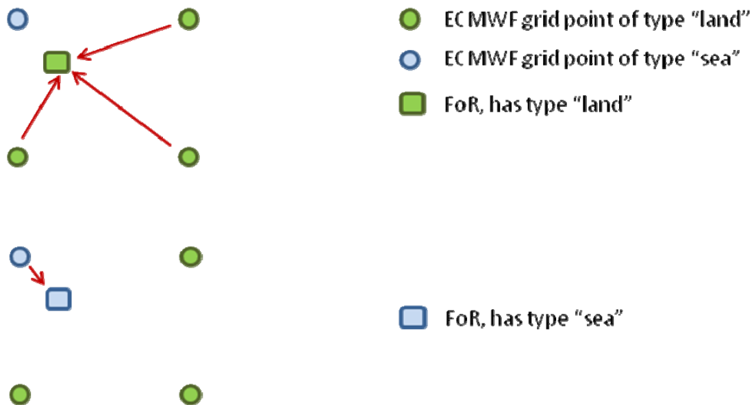
Figure 2: Schematic illustration of the use of forecast data depending on the FoR and the forecast grid surface type. Only the forecast data of the same surface type shall be used, as illustrated for the “land” case (top) and the “sea” case (bottom). The arrows denote which ECMWF grid points shall be used in these cases.
