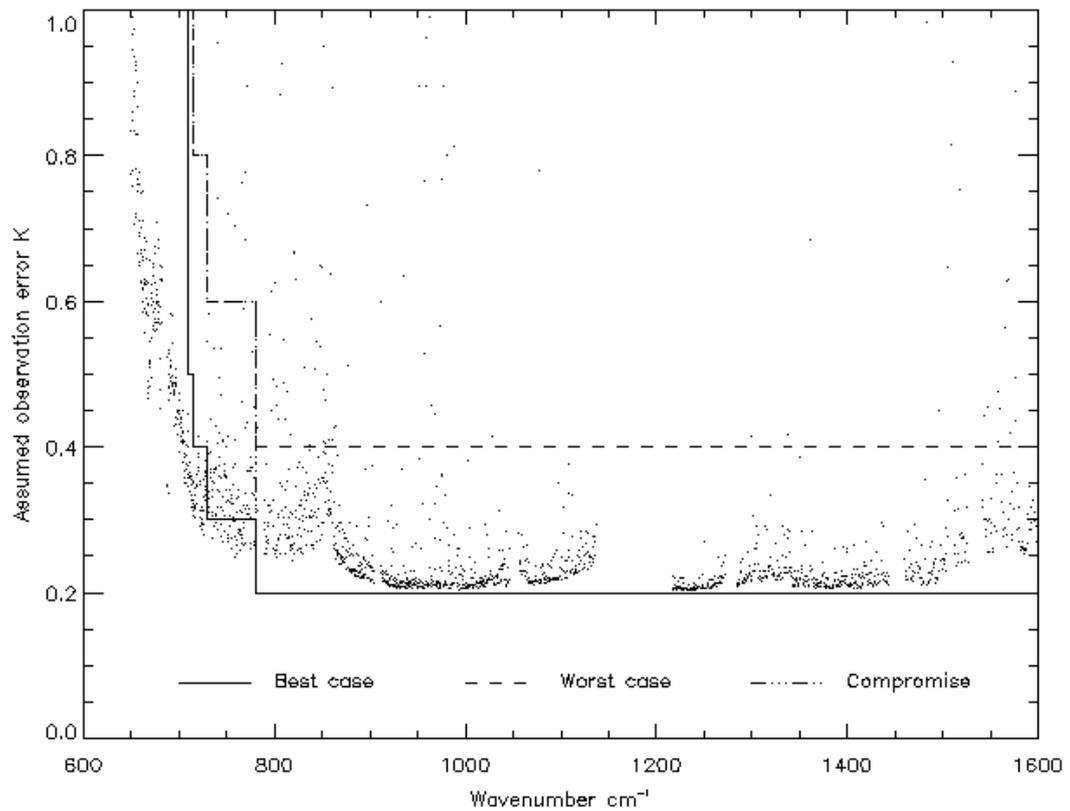
**Figure 3:** Measurement errors simulated in this study (at 280K scene temperature), compared with AIRS errors (dots). Solid line: best case (N1); Dashed line: worst case (N2); Dot-dashed line: compromise case (N3).
