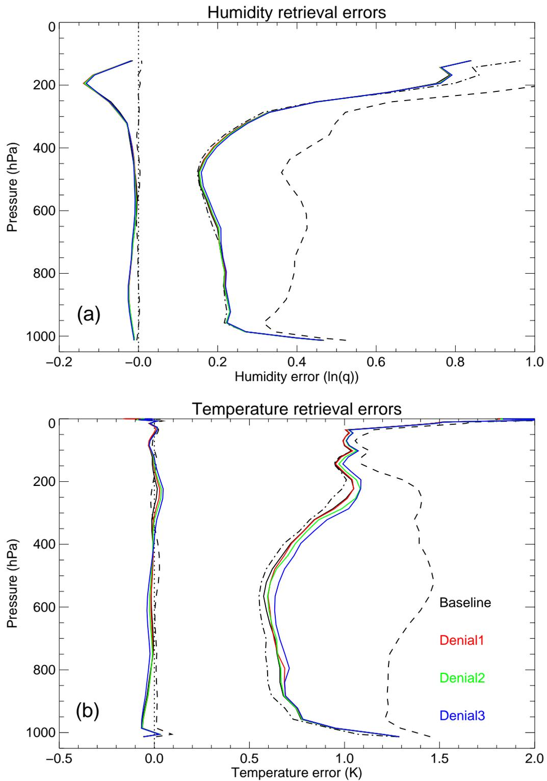
**Figure 9:** As Figure 4, but showing retrieval errors for the three CO<sub>2</sub> band data denial experiments for the N1 (best) noise case.
